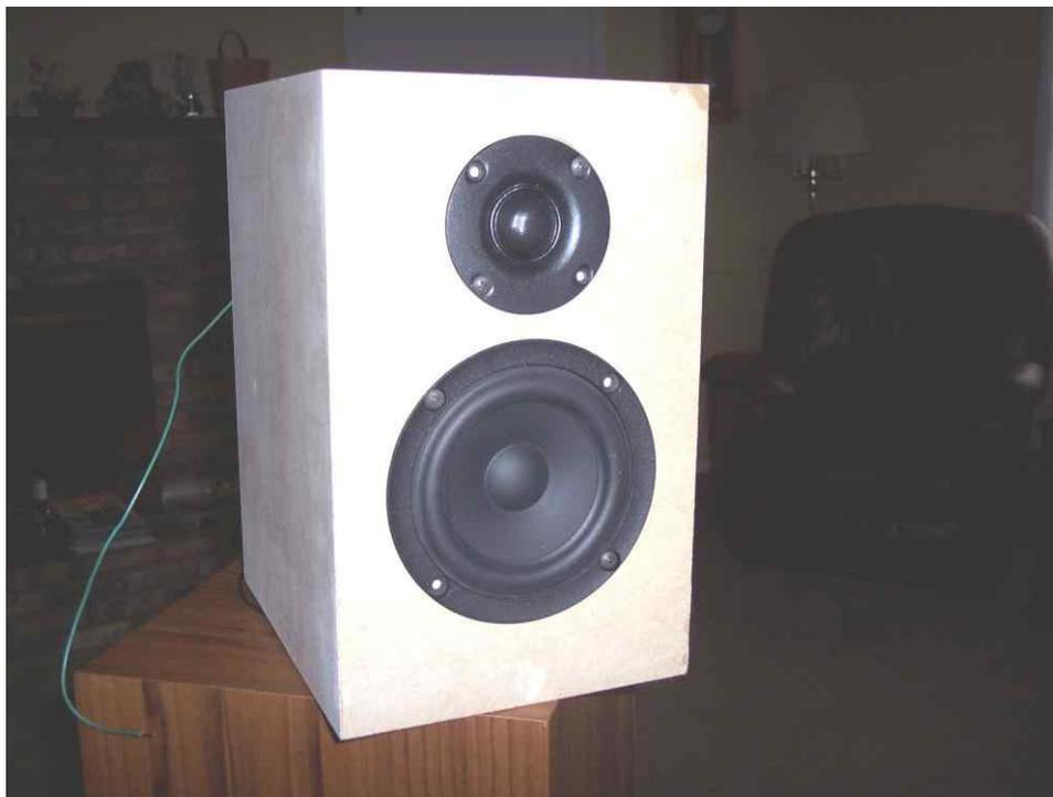
These speakers are ported on the back. I used a standard 1.25" diameter adjustable port that Meniscus sell. To make it even easier, I used only the inside section with the mounting flange. This leaves the port a little over 4" long and tunes this enclosure to 61Hz. However, since this port is adjustable I will give you some options. Here's a pic of the front and back of the finished painted enclosure.
