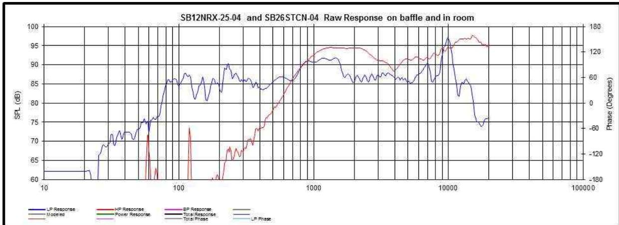
A crossover will need to deal with these diffraction affects as well as blend the drivers for a smooth, flat summation and deal with the acoustic offset as well. For those who are interested I measured the relative acoustic offset between the tweeter and midwoofer to be 17mm (woofer acoustic center behind the tweeter's acoustic center).
