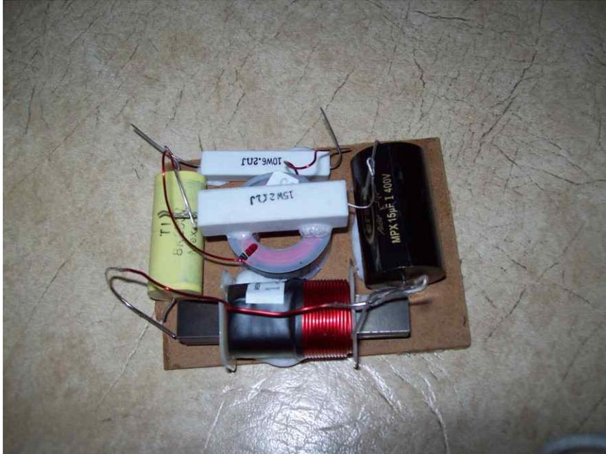
Make sure your crossover boards can fit through a hole 3.75" in diameter. Here's how I laid mine out on the board.
