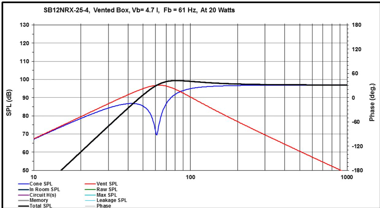
If, on the other hand, you prefer a flatter alignment then you can use both sections of the port and glue it for an overall length of 6.5". This gives you a tuning frequency of 51Hz, a -3dB point of 53.6Hz and a -6 dB point of 45 Hz, but power handling with a be little less at too. Here is a chart of that response.
