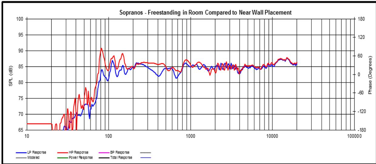
The effect of the boundary can be seen, but the design works well in either location. The dip in the response in the free-field response is similar to that of the LS3/5a and is not nearly as noticeable as you might be inclined to think, and vocals sound extremely lifelike and open from these speakers. These Sopranos really sing.
