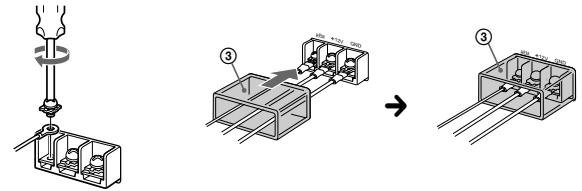
**Pass the wires through the cap, connect the wires, then cover the terminals with the cap.**
