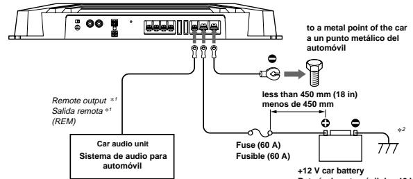
\*<sup>1</sup> If you have the factory original or some other car audio unit without a remote output for the amplifier, connect the remote input terminal (REMOTE) to the accessory power supply.
