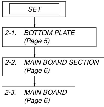
Note : Follow the disassembly procedure in the numerical order given.
