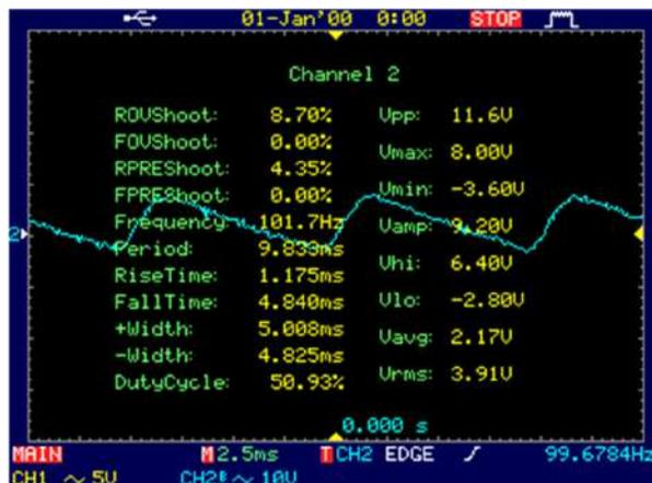
SMPS Voltage in idle is 109VDC no load, Ripple above at the SMPS output while it is LOADED **620W ==> 96.9VDC @ 6.46A** No Extra capacitors used.
