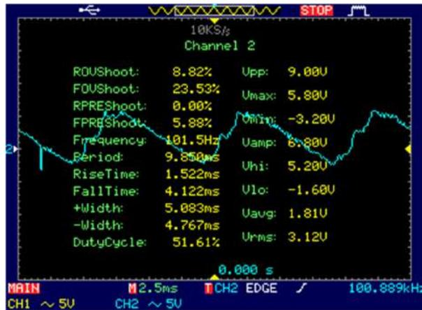
SMPS Voltage in idle is 109VDC no load, Ripple above at the SMPS output while it is LOADED **1116W ==> 90VDC @ 12.4A.**
