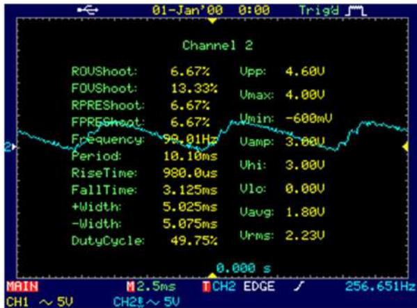
SMPS Voltage in idle is 109VDC no load, Ripple above at the SMPS output while it is LOADED **620W ==> 96.9VDC @ 6.46A**
