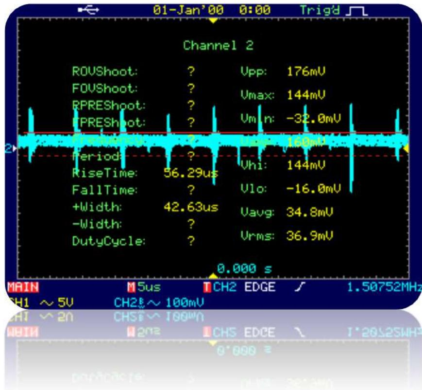
Image above is taken from **another SMPS unit**, while it's in Idle, no load at the output, spikes are clear for your reference.
