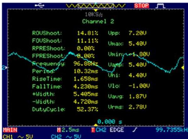
SMPS Voltage in idle is 109VDC no load, Ripple above at the SMPS output while it is LOADED **956W ==> 93VDC @ 10.29A.**
