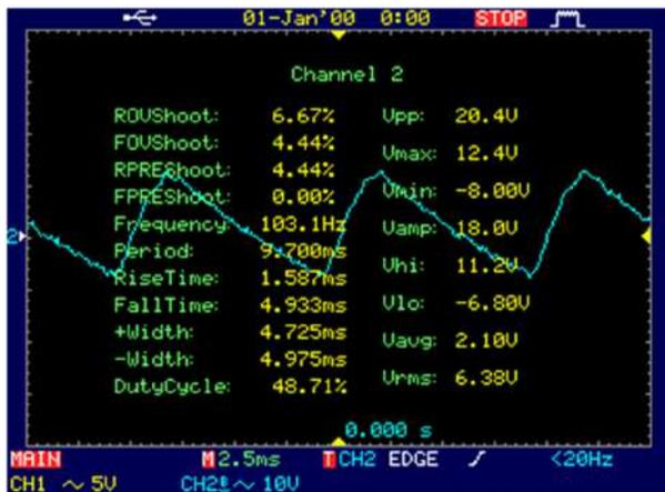
SMPS Voltage in idle is 109VDC no load, Ripple above at the SMPS output while it is LOADED **1116W ==> 90VDC @ 12.4A** No Extra capacitors used.
