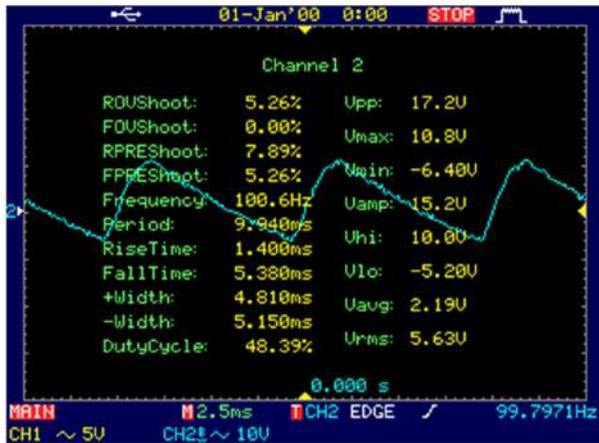
SMPS Voltage in idle is 109VDC no load, Ripple above at the SMPS output while it is LOADED **956W ==> 93VDC @ 10.29A** No Extra capacitors used.
