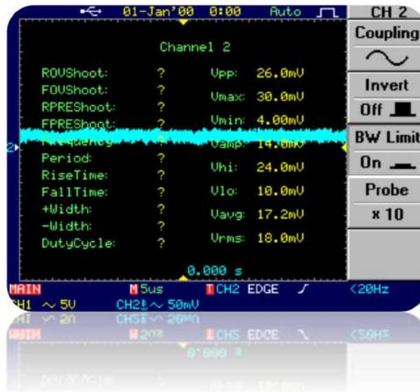
Image above is for oscilloscope noise floor, while the SMPS is completely OFF-LINE, and its capacitors are fully discharged.
