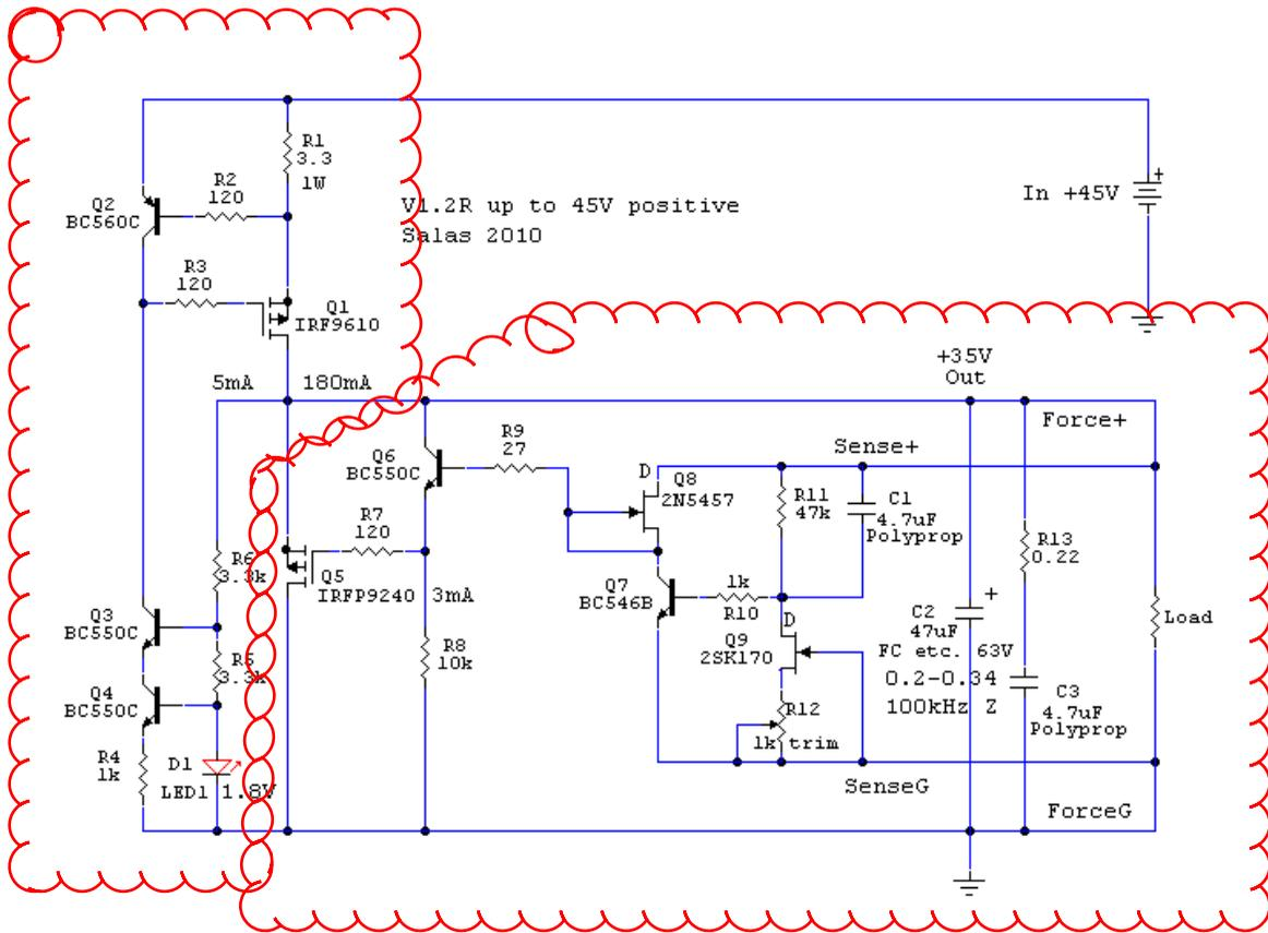
shunt + error amp x 3 according to the RIAA stages
