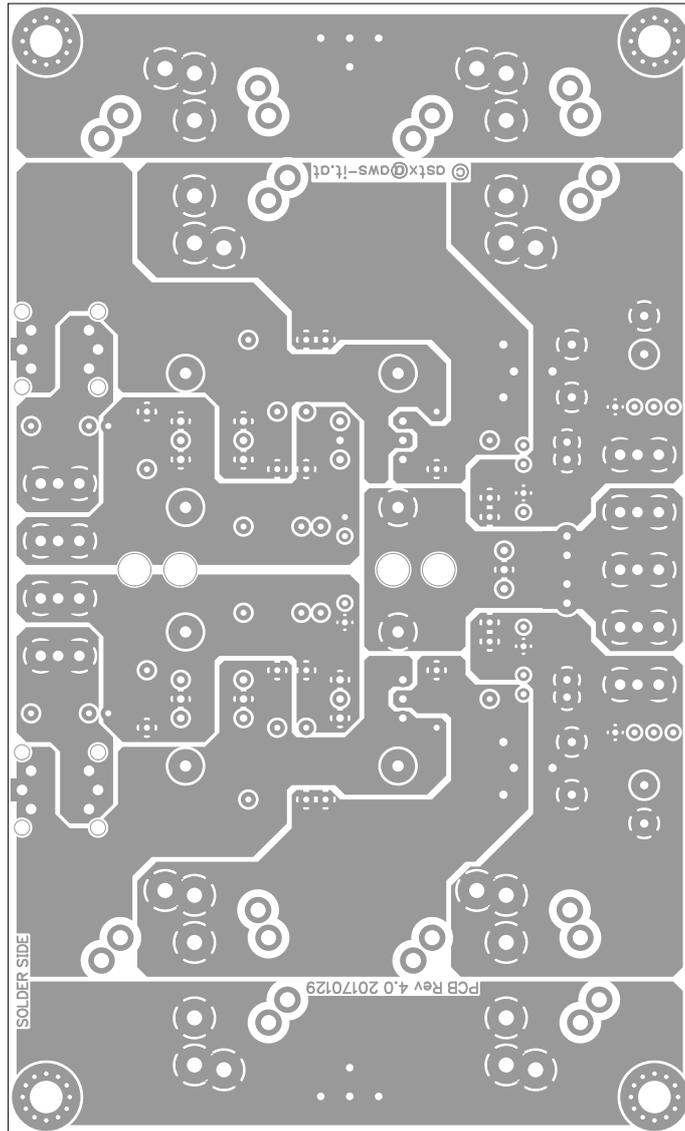
There are 8 different drill sizes used in this layout, 278 holes total
