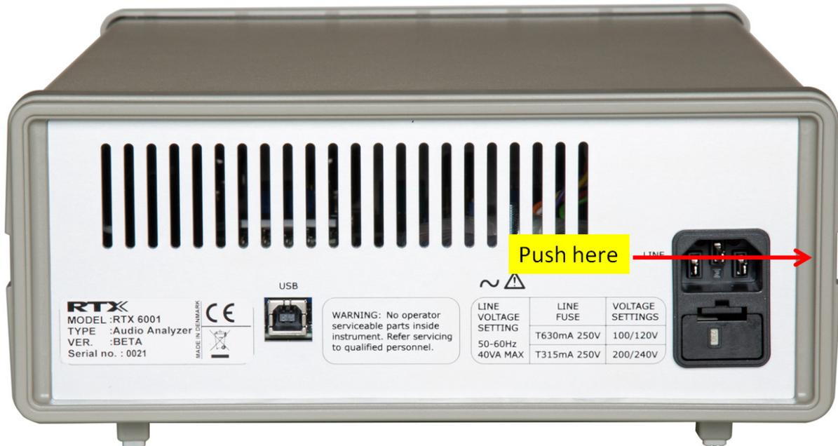
2. When pushed out to the side, move that side of the bezel away from the front/rear plate.
