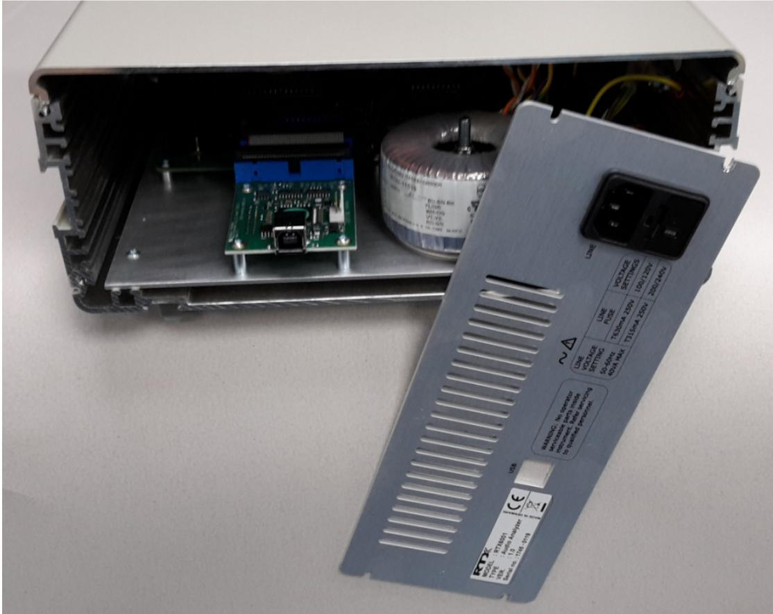
4. Remove the lid. Either by sliding it out or by using a large flat screwdriver to lever the lid as shown below. Support the screwdriver on the main chassis. Sliding the lid out can be difficult, since there is generally a very tight fit between the lid and the main chassis.
