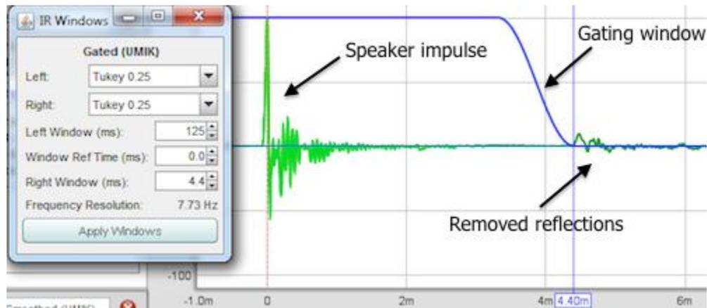
Clicking back on the **SPL & Phase** button will now show the gated measurement — that is, with the reflections removed from the frequency response calculation. Here it is (shown on the **Overlay** screen) in green:
