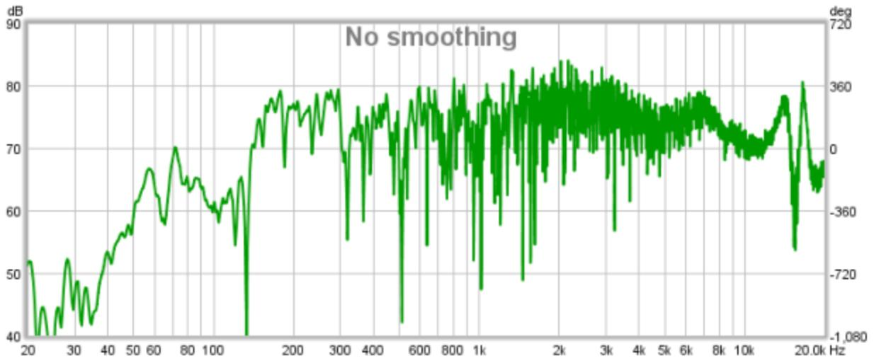
Obviously, without a little work, this is fairly hard to use! One way to address the problem is to use an anechoic chamber, which is a very large room with lots of acoustic absorption in it so there are almost no reflections. Most of us don't have one of those. Another technique is to use a *gated measurement*, where the reflections are simply removed from the measurement. We can do this in REW.
