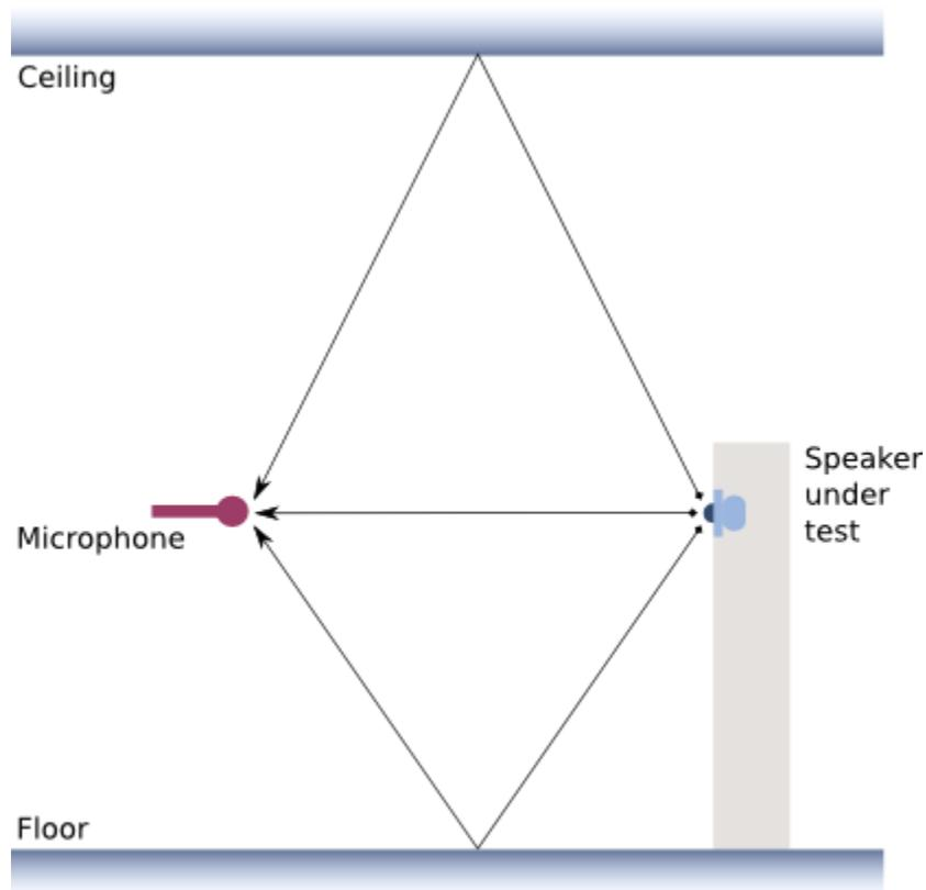
The sound from the speaker arrives at the microphone first, followed by a reflection from the floor, then from the ceiling, and somewhere along the way from the side walls. These reflections continue to bounce around the room for up to several hundred milliseconds. That is what we hear, but it makes it hard to get an accurate measurement of **just** the loudspeaker! To illustrate, here's a measurement of a 3-inch full-range driver taken with the UMIK-1 and REW in a typical domestic environment:
