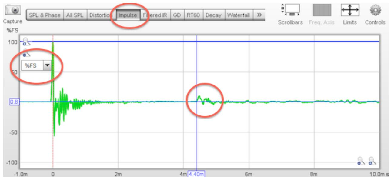
Yep! There it is... To eliminate this reflection (and all subsequent reflections), we will gate the signal at 4.4 ms as shown by the marker. Go to Tools→IR Windows, set the "Right Window" to 4.4 ms, and then click **Apply Windows**. The "window" is the region of time that REW uses to calculate the
