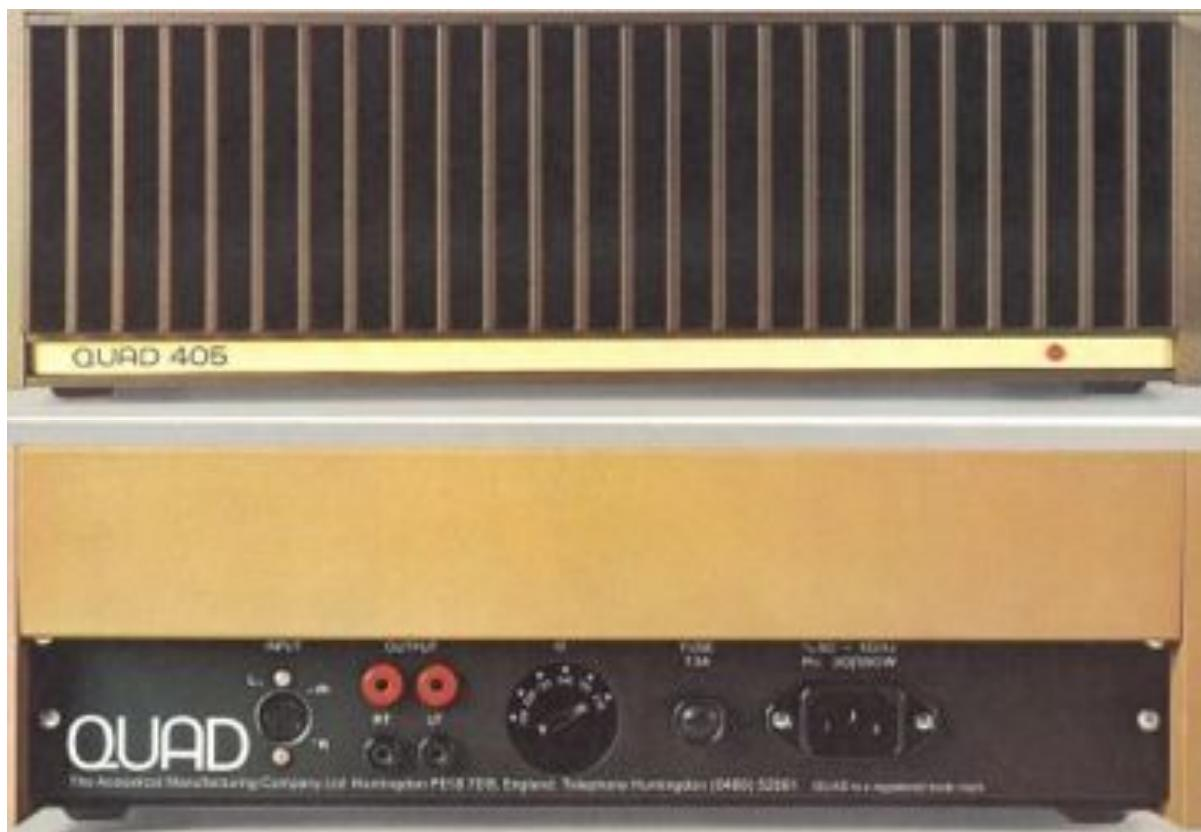
Current dumping is the name given to an entirely new audio amplifier output circuit developed by Acoustical, in which the majority of the main current carrying transistors (the current dumpers) has no bearing on the overall amplifier performance, thus the need for bypassing and allied problems associated with crossover are eliminated.
