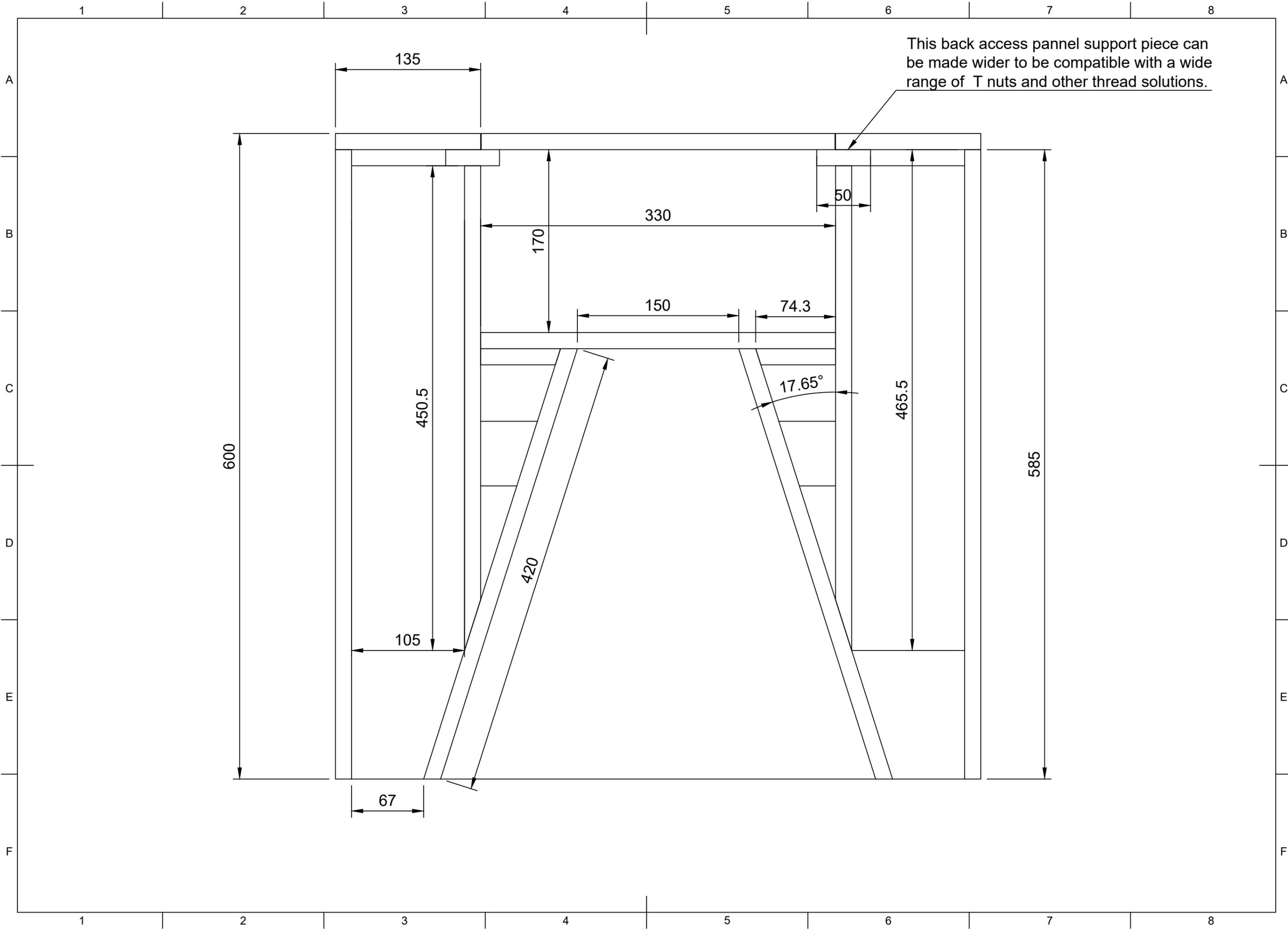
This back access pannel support piece can be made wider to be compatible with a wide range of T nuts and other thread solutions.
