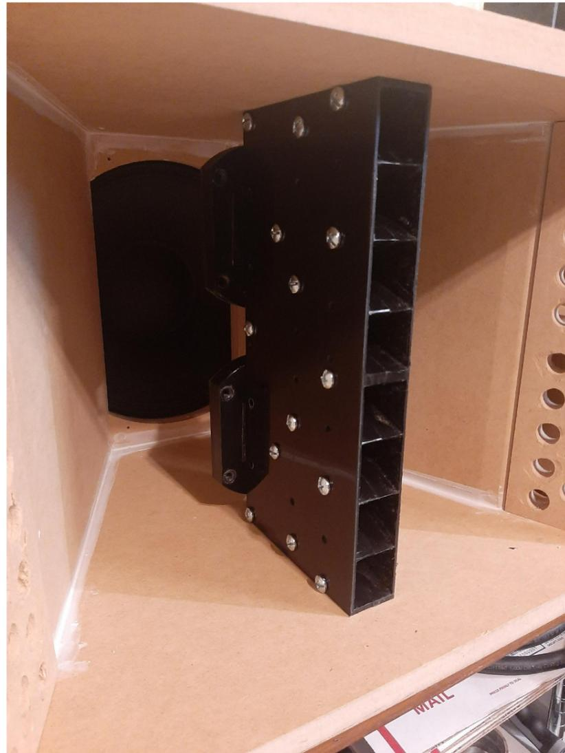
Lewis Cafaro has developed a series of custom made line-array style waveguides which are time aligned specifically for Paraflex tops.. This means that when using such a waveguide the HF and LF elements of the cabinet are readily aligned in terms of phase & time so it is not necessary in DSP to apply additional delay to the HF compression driver (meaning no need to add more delay than you have on the 12" driver's DSP channel) ....
