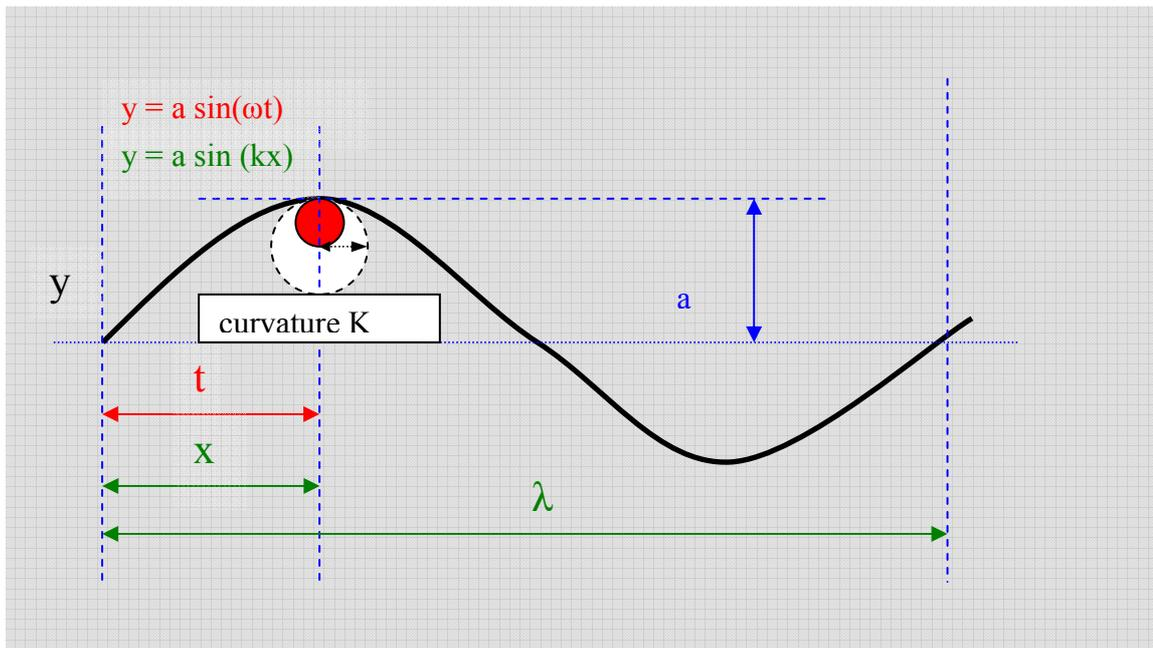
Groove lateral position  $y$  [m] described in two systems, time and position :
