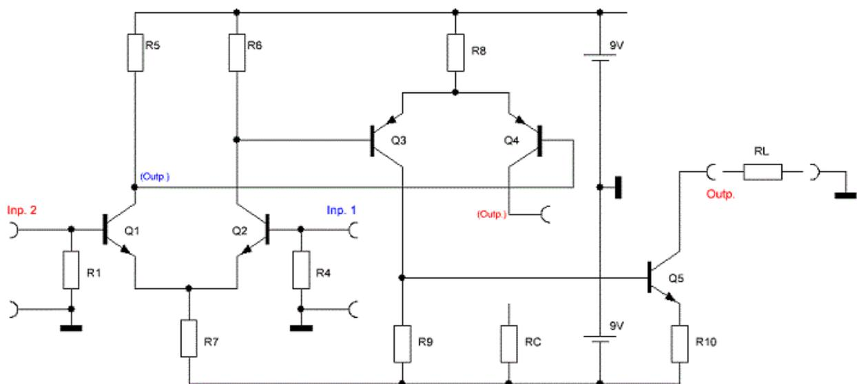
In other words, the symmetrical bridge voltage must be related (as one voltage) to ground. We should be able to add both opposing output voltages; with the result  $Y_+(x)$  plus  $Y_-(x)$  equal zero,  $Y_+(x)$  minus  $Y_-(x)$  leads to 2 times  $Y(x)$ . An automatic gain of 6dB!
