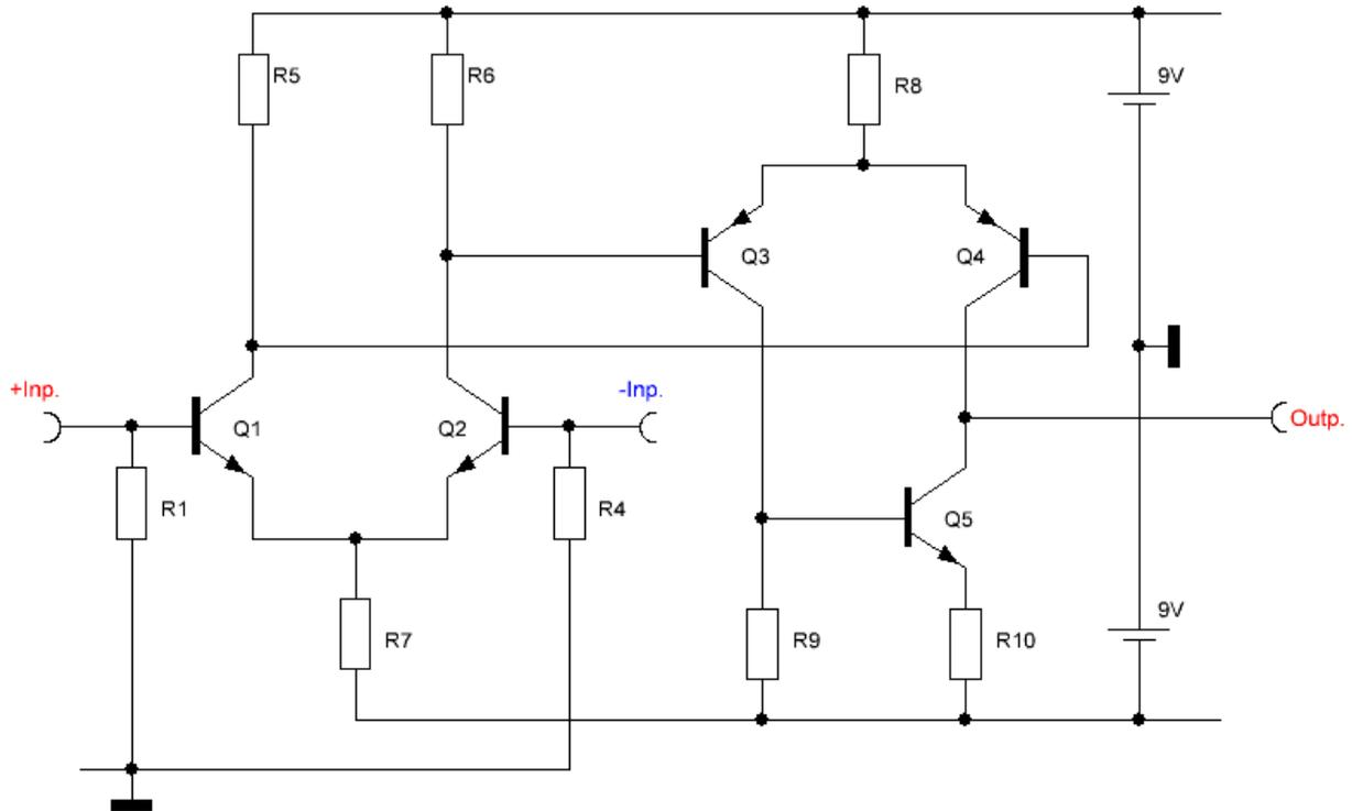
As soon as we realize that both collectors with their conducted potential will move in the same direction under a signal modulation, we can consequently also connect both electrodes with each other - especially since the same currents, even one and the same one, are flowing.
