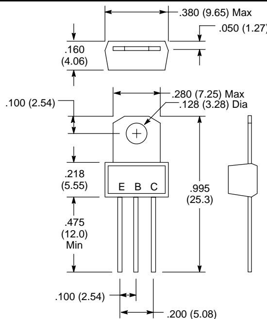
Collector Connected to Tab
