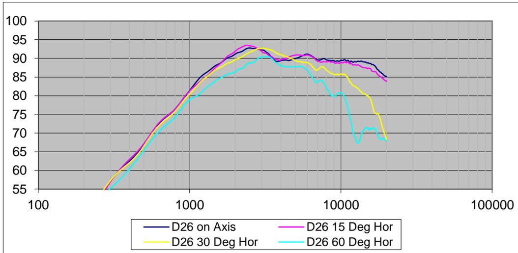
Like the woofer, the two tweeters were nearly identical in response (in box before eq).
