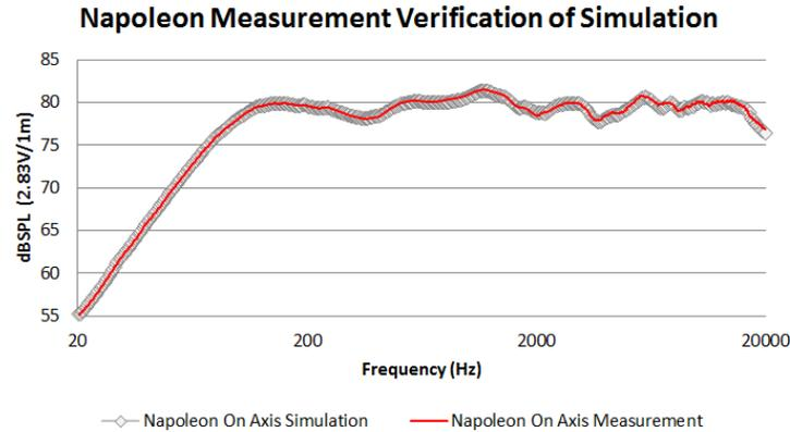
These can be considered highly accurate reflection-free responses. All sensitivities following are at 1 meter, 2.83V. Measurements were taken in 15 degree increments 0 to 90 degrees off axis horizontal, and 0 & 15 degrees off axis vertical to be used in crossover design. A few examples follow to help explain some of the crossover choices made.
