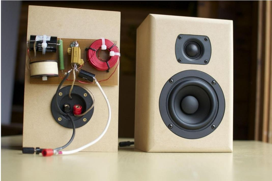
The Napoleons are a small DIY loudspeaker designed to deliver a natural tonal balance and clean loud playback from of a small box optimized for small reflective rooms, but still perform well in larger spaces, at a reasonable price. This write up was in response to requests from the 2013 Ottawa DIY fest, where the speaker was first shown <http://www.diyaudio.com/forums/clubs-events/223294-diy-ottawa-winter-2013-a-17.html>
