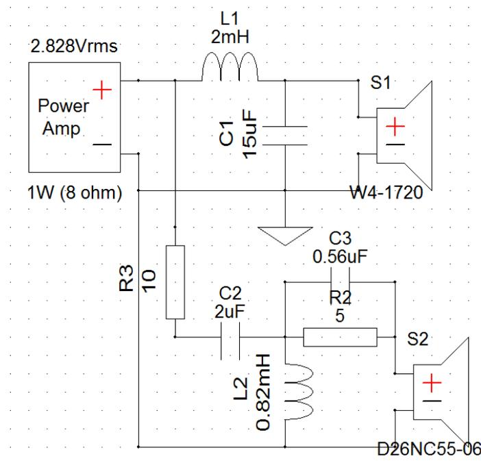
No special treatment for low inductance resistors is necessary. For example, the inductance of a Vishay RH-25 was found to reduce 10 kHz by only 0.03 dB.
