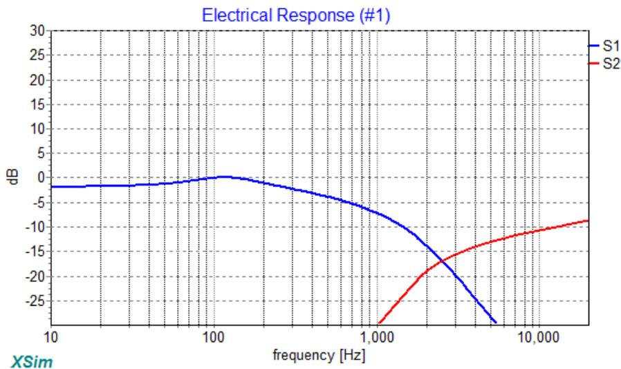
Electrical System Impedance is an easy drive even for chip amps as it never dips below 5 ohms, and never gets too capacitive.
