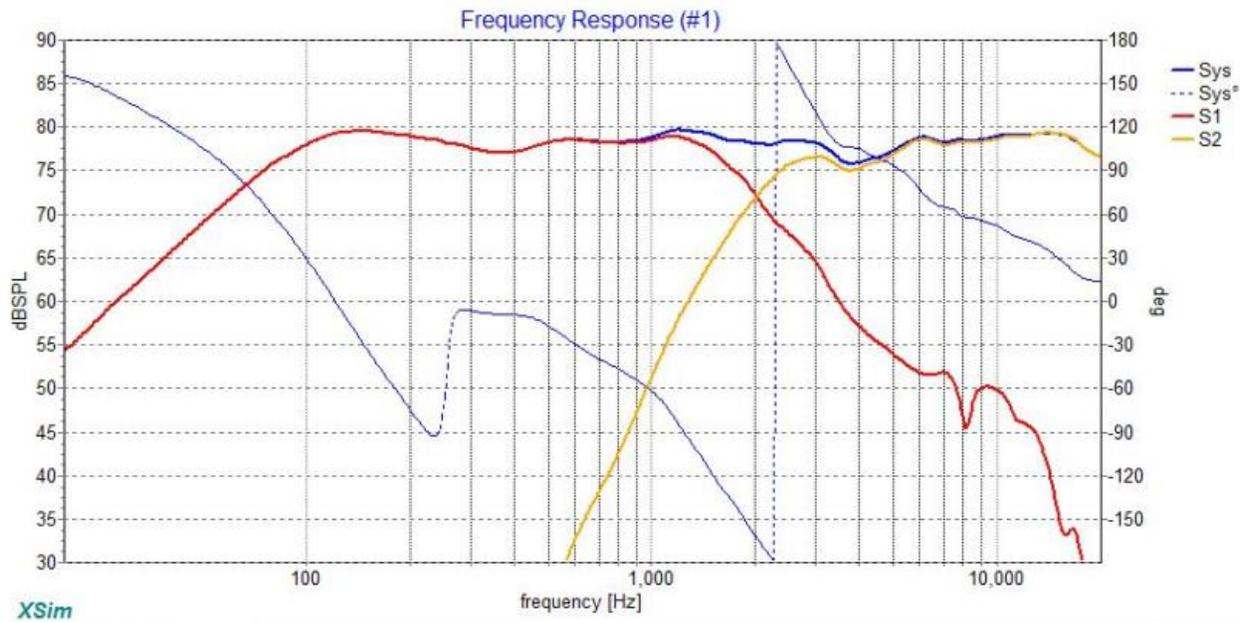
The following illustrates the differences on axis between this crossover and the previous iteration as found in Appendix II. “#2” is previous iteration, “#3” is this crossover.
