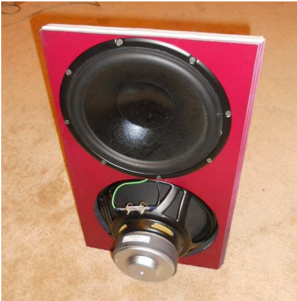
Woofers mounted on baffle.
