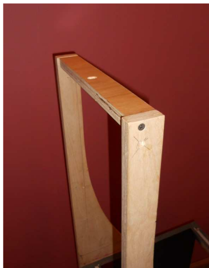
Top baffle brace positioned between side panels and secured with screws.
