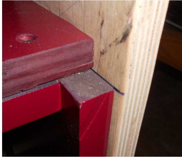
Step at front of woofer enclosure which main baffle rest on.
