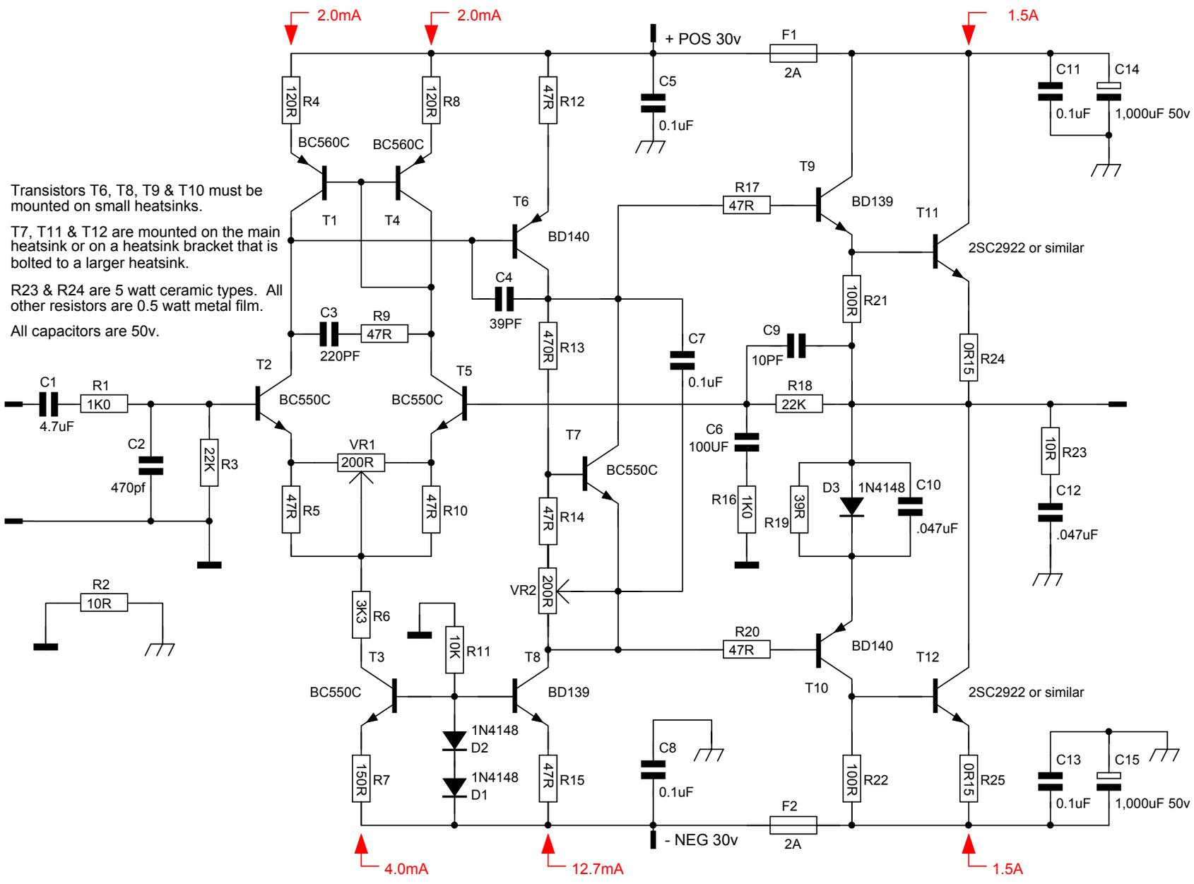
Transistors T6, T8, T9 & T10 must be mounted on small heatsinks.
