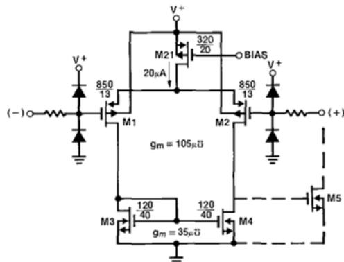
FIGURE 1—Input stage with common-mode voltage range that includes ground.
