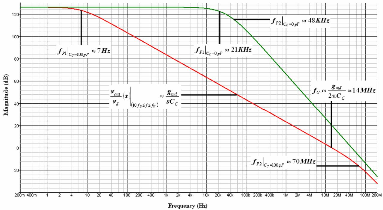
**Figure A4.** The apparent migration of dominant poles due to Miller-effect compensation on the forward path's frequency response (red trace). The green trace represents the uncompensated forward path's frequency response.
