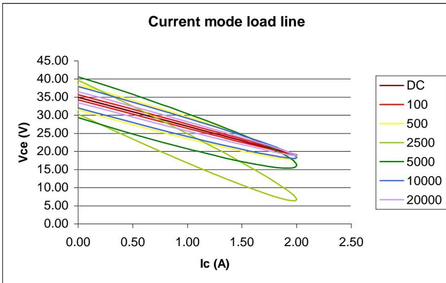
Though load modulus and phase angle may be computed solving the circuit, it is more handy to draw and simulate it and read out values for the selected frequencies.
