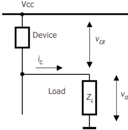
With reference to the actual operating condition for non resistive loads, with an eye to its impact on SOA, looking at the simplified schematic above we may write for the positive going quadrant:
