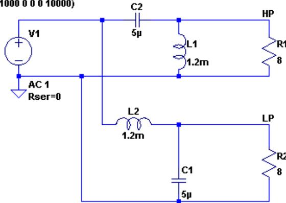
This is a highly simplified 2-way second order passive 2 kHz crossover network, where the drivers themselves are replaced by ideal resistive loads, something that is not true, yet the reactive frequency dependent load impedance nature is present. In an actual situation, load impedance frequency dependence is more complex but not very different qualitatively.
