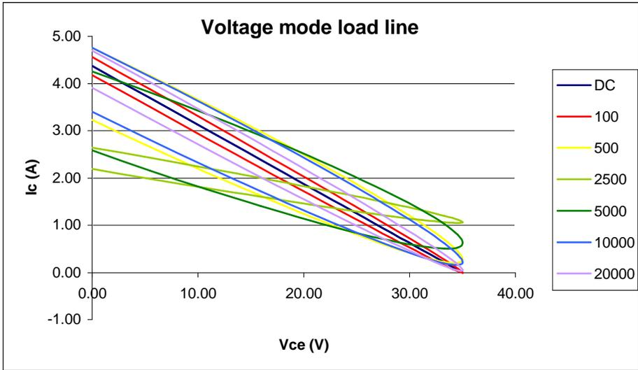
At left is the corresponding plot for voltage mode as given by [4]. Again note the dependency on combination of voltage slope and phase angle sign. To read this plot in reference to SOA verification, it must be rotated and mirrored so
