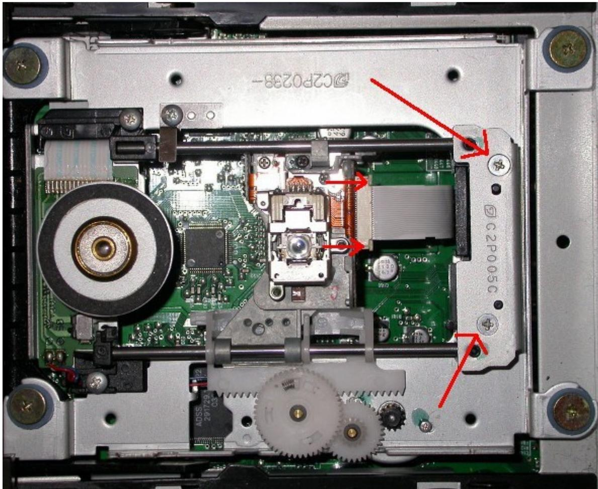
4. Push the laser pickup in this direction and replace it with the **unsoldered** new pickup.
