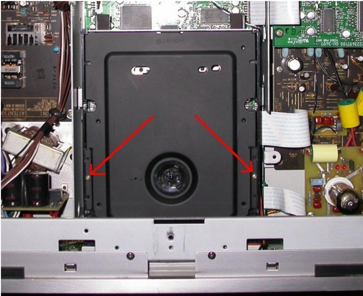
3. Deattach the back white flat cable and remove the two screws:
