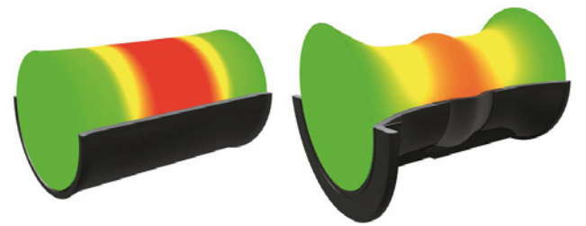
Figure 43. Pressure of the first resonance in a port with rigid walls (top) and flexible walls (bottom)
