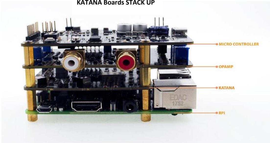
The KATANA stack consists of 3 boards plugged into the 40 pin GPIO header of the RPI.
