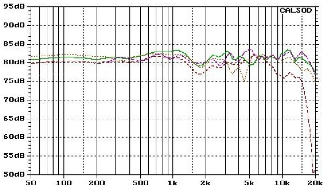
The crossover uses a broad overlap between woofer and tweeter but with tweeter high pass high enough in frequency to avoid tweeter distortion when pushed hard.
