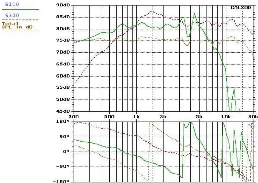
Ideally, these resonances would be suppressed by 25 dB or more, but it quickly became apparent that this would necessitate higher order filters. This wasn't pursued in order to minimize the filter order; my preference is to allow as much overlap as possible, within the constraints of the off axis response and driver power handling, as it is felt this better blends the tweeter's off axis dispersion through the crossover frequencies, with the woofer's.
