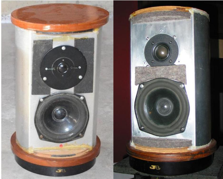
Felt was placed at the end caps and above the woofer to minimize unwanted reflections (which show up in JR's measurements for the original) that would harm the frequency response and the imaging. McMaster Carr F-13 Felt in 1/2" thickness was used. The strip between the woofer and tweeter was found through measurement to remove +/- 1 dB peaks and nulls on axis from approximately 2 kHz to 5 kHz, by reducing tweeter diffraction off the woofer cone.
