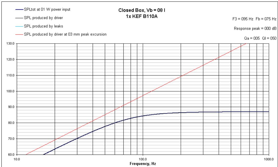
Note that the above curve is deceiving as it accounts for neither voice coil inductance, nor the high pass effect of diffraction as the cabinet changes its radiation from half-space to full space. This will be shown in measurements which will follow.
