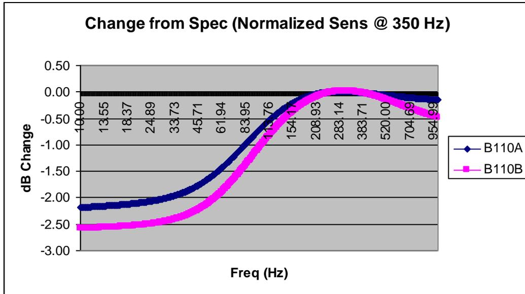
The impact was less than 1 dB above 83 Hz, and 2 dB at 61 Hz. Given the limited range of the B110 below 80 Hz, the impact wasn't a showstopper. In absolute terms, the variation is within the range of room placement variance, and the design parameters provided an over-damped response, per the intent of the original:
