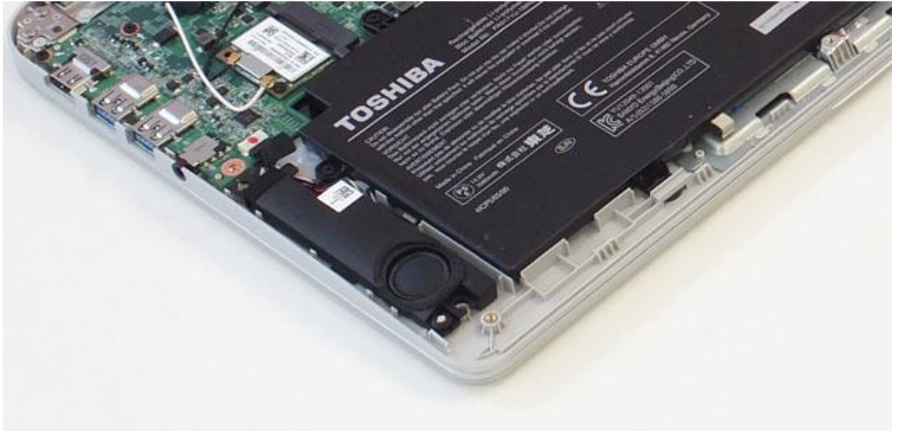
Small speakers are never going to deliver a significant bass response
