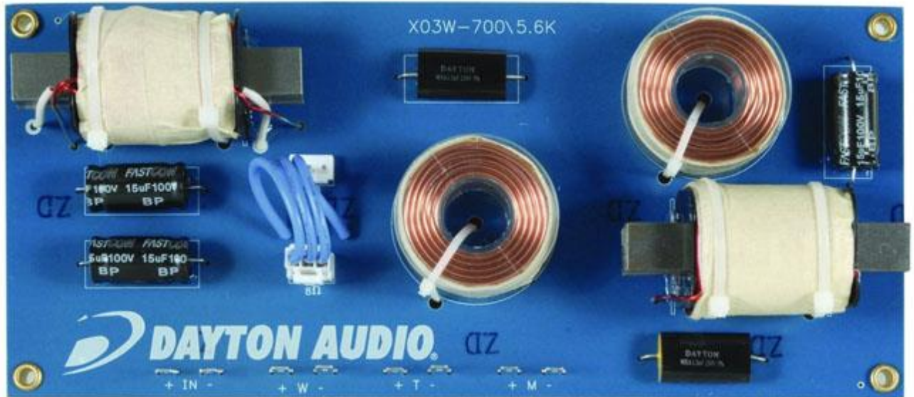
Passive crossover designs abound but will always have inherent delays
