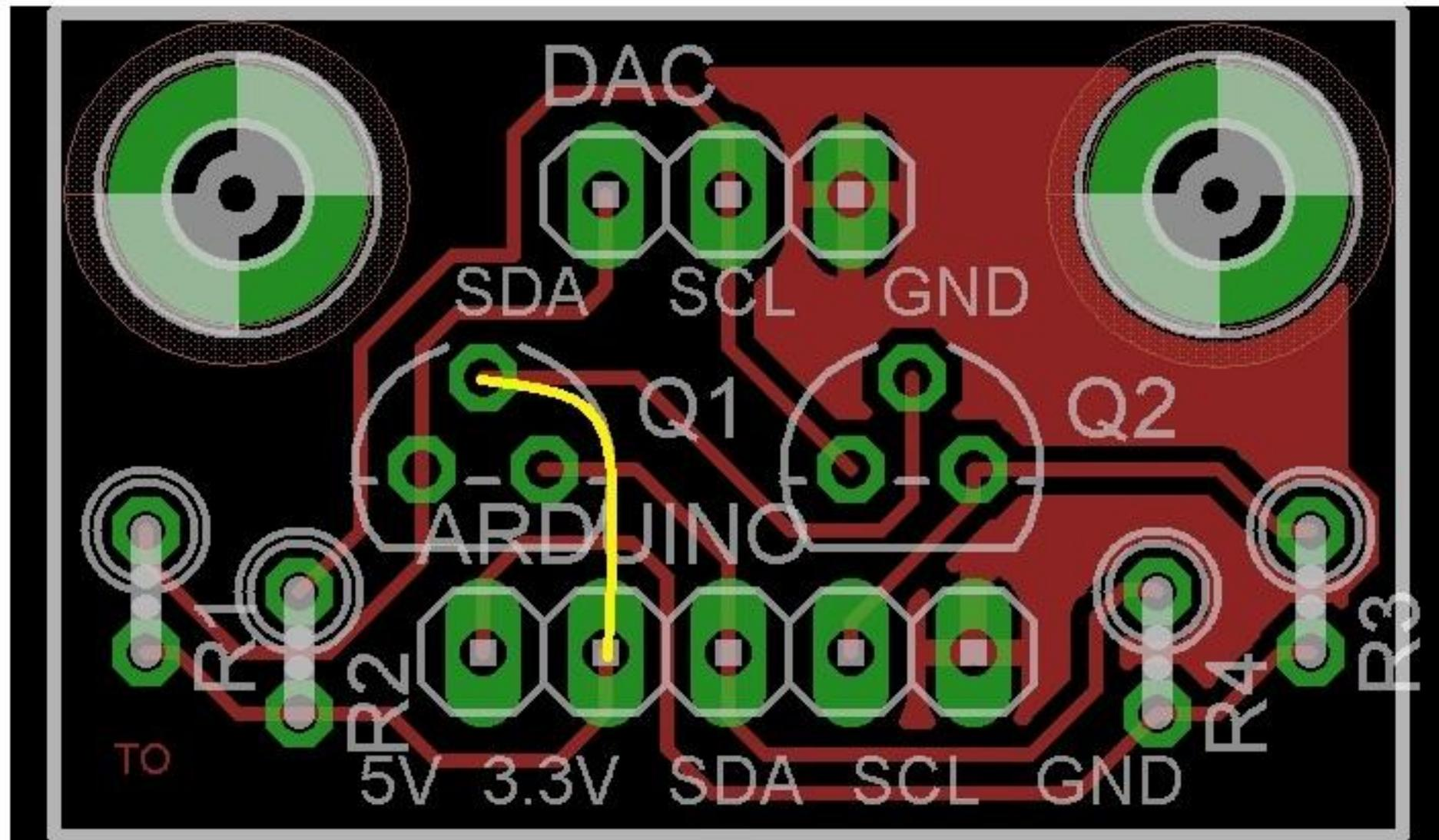
**Note:** Connect the two points 3.3v and gate of the FET as shown in yellow using a wire on the bottom side of the board . Also note that the legends printed on this level shifter board is printed on the back side by mistake. So the side which is not printed is actually the top side. You can use this picture as a reference for soldering. This picture is actually the top side of the level shifter board.
