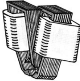
"POLE PIECE STACK" ASSEMBLY
