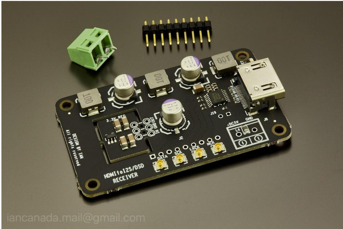
2. HDMIpi PCM/DSD/DoP receiver with HDMI cable
