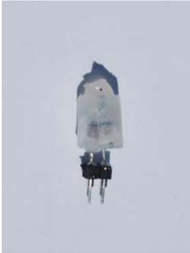
*In doing this final step, first use squeeze some silicone compound within the tubing, before applying it over and around the GLED431 circuit. This step surrounds and isolates D1/Q1 within the silicon, as well as holds the tubing in place, once the silicon has set up.*
