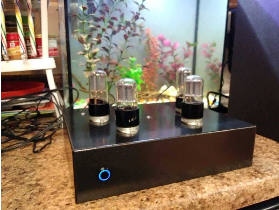
A picture of the original prototype of the Flea Amplifier, with Russian surplus 6N9S and 6N8S tubes installed.
