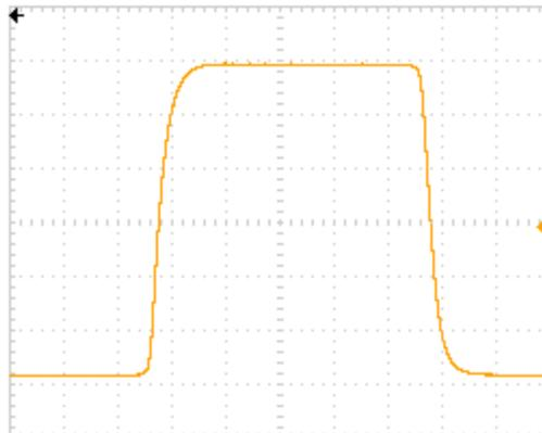
The amplifier takes advantage of the square law character of Field Effect Transistors to have a graceful transition from the Class A region for a wide range of bias levels, even when presented with high current into lower impedance. Here is the current waveform experienced by one half of the output stage as it approaches shutoff at 50 watt peak into 8 ohms:
