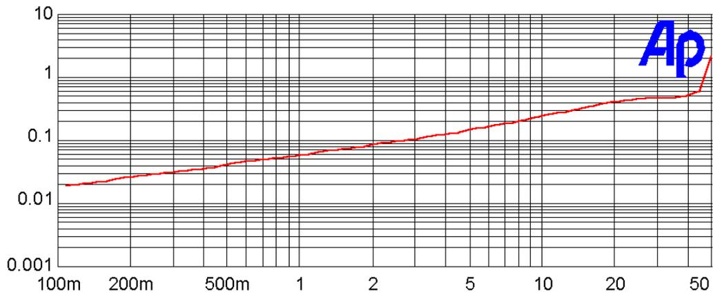
And distortion vs frequency at 1 watt, 8 ohms:
