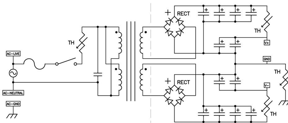
The power Thermistors are used to suppress inrush at turn-on and also as RC filters on the capacitor banks to lower the noise on the rails seen by the channels. Also a Thermistor is useful for connecting circuit ground to chassis when you are trying to avoid ground loops while still maintaining a safety earth connection. The AC line fuse would be chosen at a rating lower than the current rating of the Thermistors.
