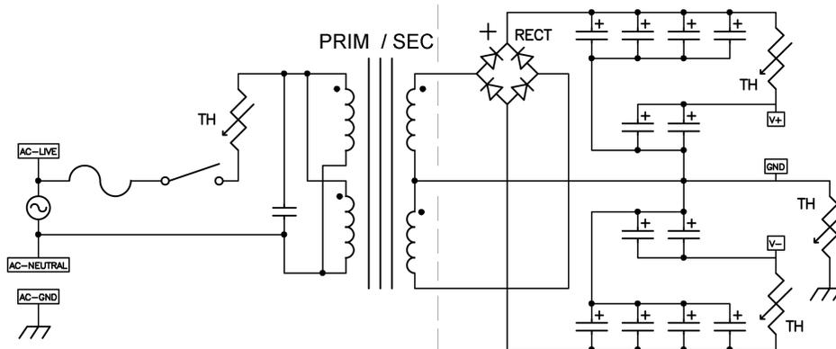
Note that the dots on the transformer coils indicate the phase of the coil, and the leads should be color coded. Take special care to not confuse the primary windings with the secondaries. Your transformer should come with some clear documentation on these connections.
