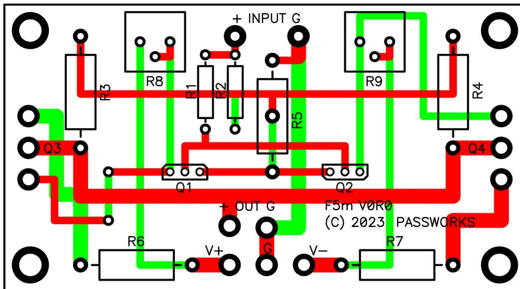
The output transistors Q3 and Q4 mount to the sink and circuit board. The board and power transistor mounts match the UMS standard for kits from the diyAudio store, but you can actually ignore the four mounting holes, as the power transistors are capable of holding the board up by themselves. Not that I recommend that..
