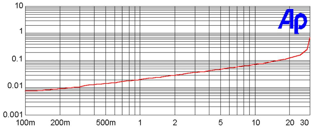
And below is the curve into 4 ohms:
