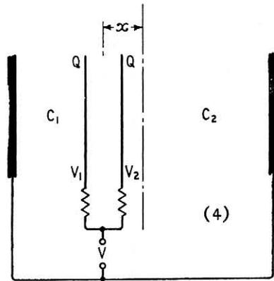
$$V_1 = \frac{Q(d-x)}{\kappa A} \quad V_2 = \frac{Q(d+x)}{\kappa A}$$
