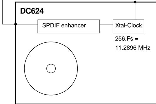
The noisy SPDIF signal in the CD624 transport could be enhanced as well.
