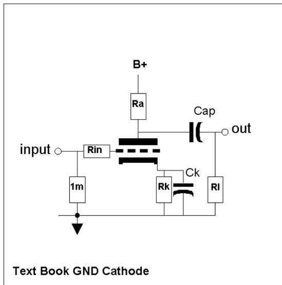
The textbook Grounded Cathode Amplifier. The most common and easiest of tube circuits. The triode is cathode biased. The output is phase inverted. The gain never exceeds the mu of the triode. Still, a very good line stage can be made from this circuit.
