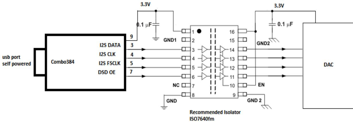
Fig.1 - Isolator between the module and the DAC.
