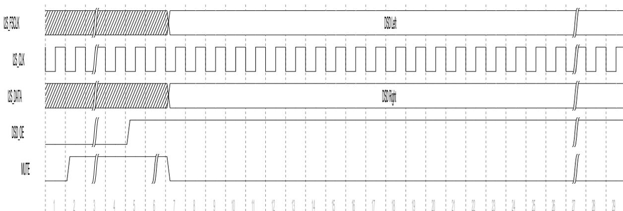
In DSD Mode the I2S\_CLK becomes the DSD clock signal, the I2S\_FSCLK becomes the output data line DSD1 and I2S\_Data becomes the DSD2 Line.
