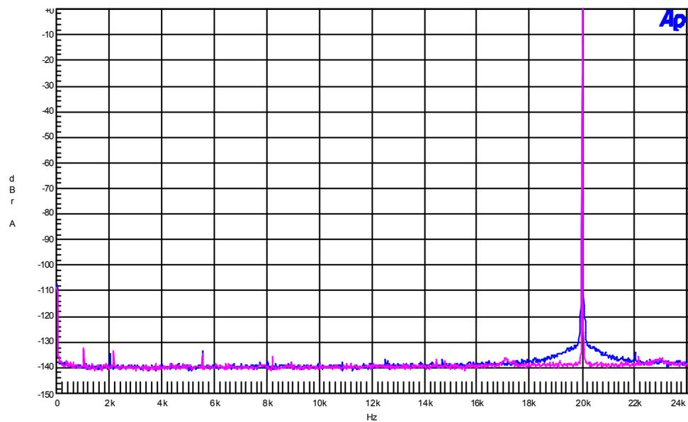
Audio Precision, Jitter susceptibility, sampling jitter using a DAC. S6k and DAC in clock master mode (lower trace) and in clock slave mode (upper trace). No jitter was applied on reference clock. Same as Figure 4.
