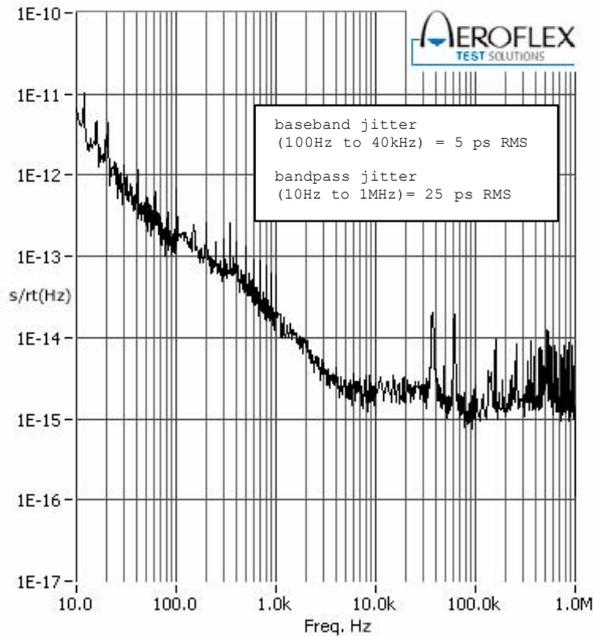
Jitter spectral density. TC Electronic System 6000, clock master mode, carrier 12.228 MHz.
