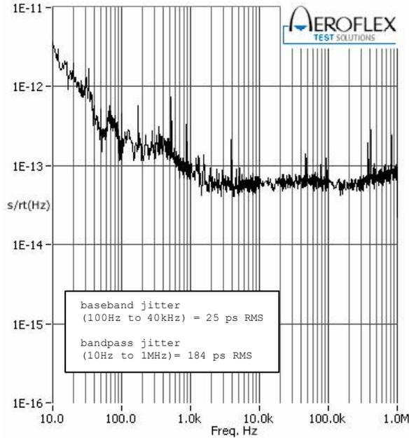
Jitter spectral density. JET on-chip VCO, clock master mode, carrier 24.576 MHz.
