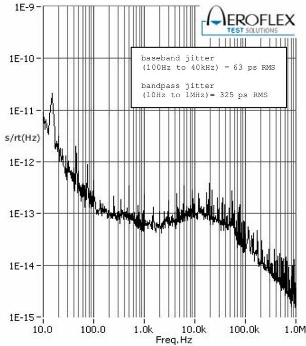
Jitter spectral density. Clock product A, DDS design, clock slave mode, carrier 12.228 MHz. No jitter was applied on reference clock
