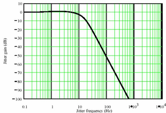
Figure 3 Jitter Transfer Function of JET when the bandwidth is set to 10 Hz.
