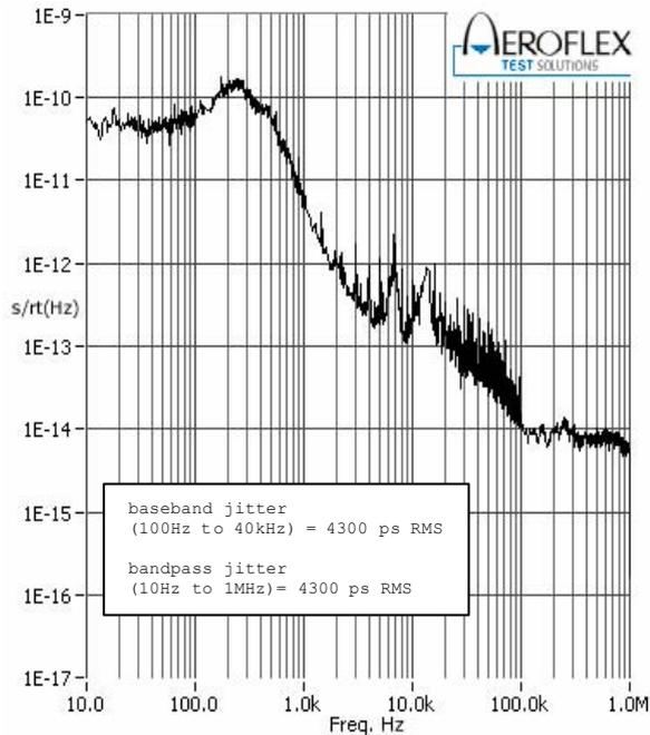
Jitter spectral density. Typical audio product, clock slave mode, carrier 12.228 MHz. No jitter was applied on reference clock. Same as Figure 8.
