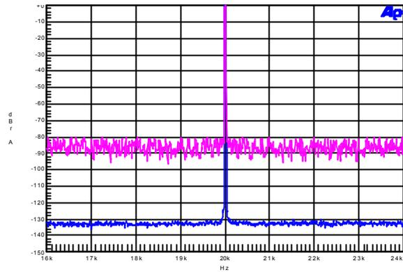
Figure 1 DAC in clock master mode (lower trace) and clock slave mode with 25 ns peak wide band jitter applied (upper trace).
