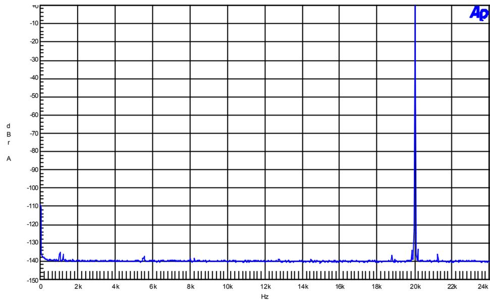
Audio Precision, Jitter susceptibility, sampling jitter using a DAC. JET and DAC, in clock slave mode. No jitter was applied on reference clock. Same as Figure 5.
