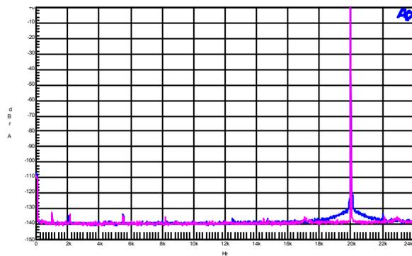
Figure 4 System 6000 DAC, in clock master mode (lower trace) and in clock slave mode (upper trace). No jitter was applied on reference clock.
