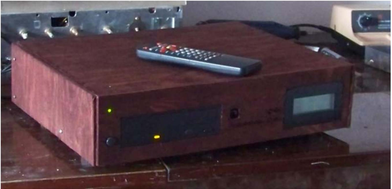
If you have flashed IC and assembled everything together, you need to test your RC-5 remote control, keyboard and display to work properly. Set the right contrast and optionally change resistors for backlight and LED to achieve the best brightness.
