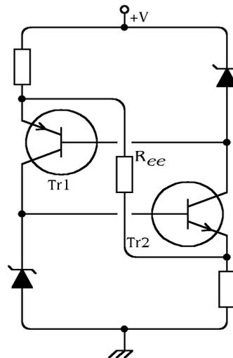
A change of voltage  $+ΔV$  will cause a current change of  $+ΔV/R_{ee}$  to flow through this resistor, but each transistor will then pass this amount less current. The net effect is that the original voltage change causes a current change of
