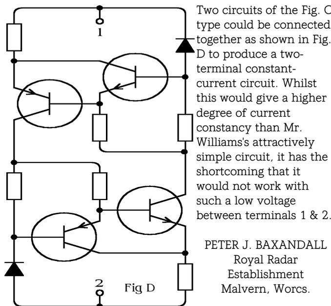
Two circuits of the Fig. C type could be connected together as shown in Fig. D to produce a two-terminal constant-current circuit. Whilst this would give a higher degree of current constancy than Mr. Williams's attractively simple circuit, it has the shortcoming that it would not work with such a low voltage between terminals 1 & 2.
