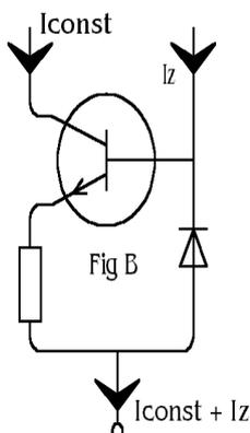
Once the Zener diodes are conducting, it seems to me that the circuit is best regarded simply as a combination of the simple constant-current circuit of Fig. B with a complementary version of the same circuit, the constant current of each circuit being used to energize the Zener diode of the other. The total constant current of the complete circuit is the sum of the constant currents of the individual circuits, which need not necessarily be equal.
