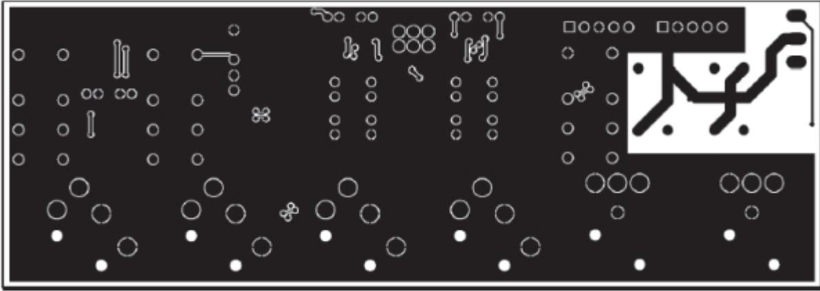
**Figure 26b: PCB bottom copper**
