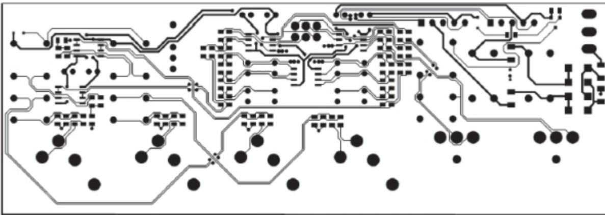
**Figure 26c: PCB top copper**
