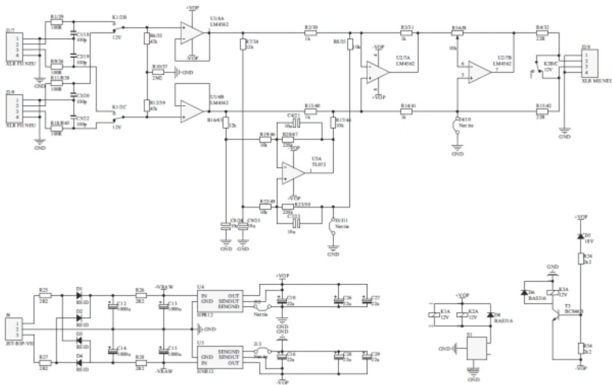
**Figure 25: Complete balanced preamp/volume controller**
