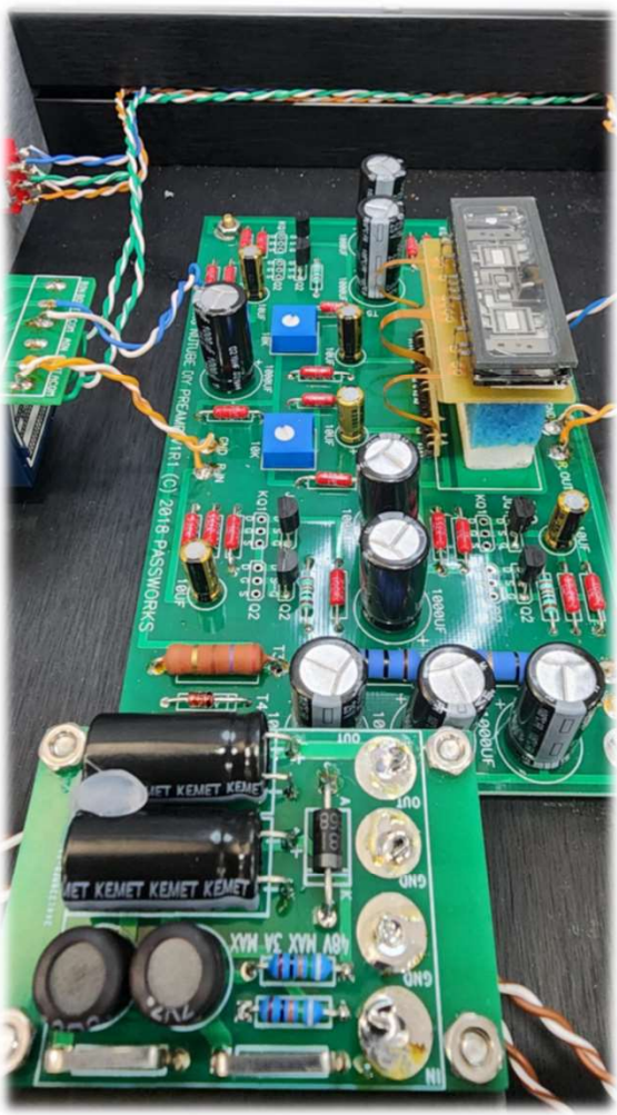
Installing SMPS Filter Board by "birdbox" • 3D Printed the mount board • Sanded lightly to tolerance fit in rail • Put M3x12 bolts from bottom up, added nylon nuts on top • Soldered wiring to SMPS board • Installed board on M3 bolts with basic nuts.
