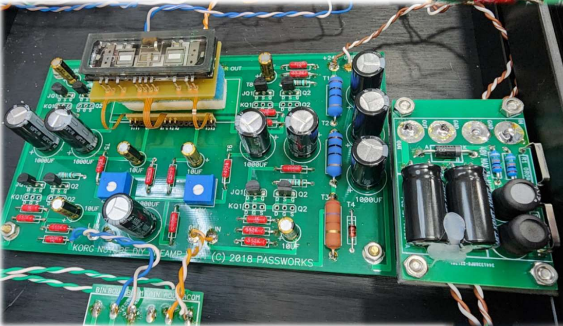
Installing SMPS Filter Board by "birdbox" • 3D Printed the mount board • Sanded lightly to tolerance fit in rail • Put M3x12 bolts from bottom up, added nylon nuts on top • Soldered wiring to SMPS board • Installed board on M3 bolts with basic nuts.
