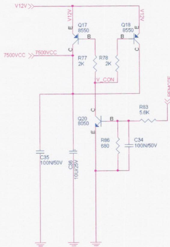
Fig.1 controlled +12V power supply circuit
