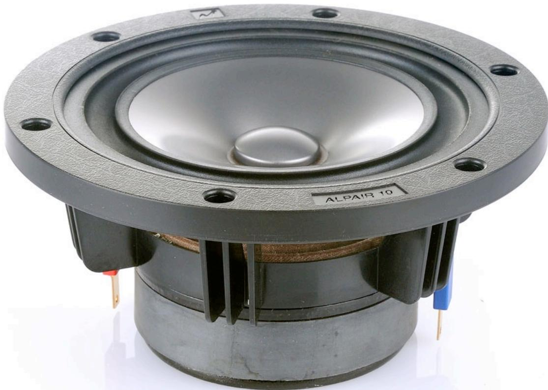
This Alpair 10 is the latest model in a development line designed to extend the performance of mid-sized Markaudio full-range emitters. Measured performance is extended.  $V_{as}$  increases from 21 to 28 litres.  $F_0$  is now 36Hz, 4Hz lower than the old model. Total Q increases to 0.33 making this new Alpair 10 usable in larger audio applications.
