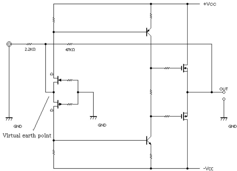
This is basic current feedback bak circuit .
