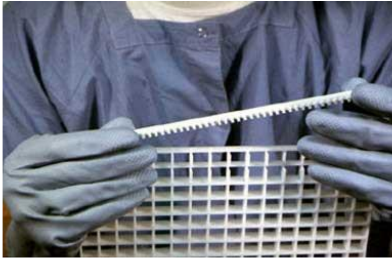
The plastic louver structure has already been trimmed to size and the ends notched to clear the wires. A custom-molded "comb" is being glued to each end of the louver. This "comb" forms the hooks to hold the wires.
