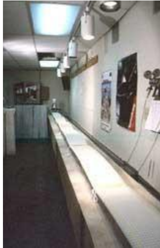
A view of the gluing track, where "Maybelline" does her thing. A vacuum system below the track pulls away the glue fumes.
