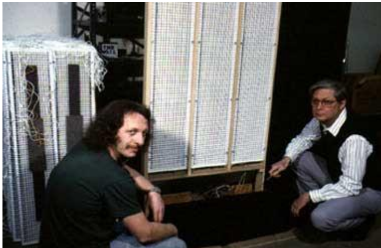
After the panels are wired, a quick acoustic check is made over a wide frequency range. This checks for any extraneous noises caused by loose Mylar or foreign objects trapped in the panel.
