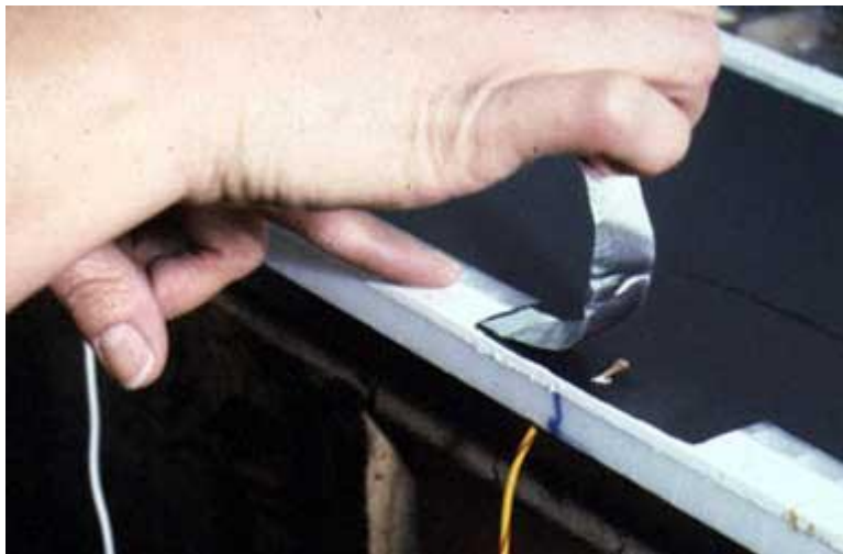
The bias feed wire is attached, and held in place with self-adhesive foil tape.
