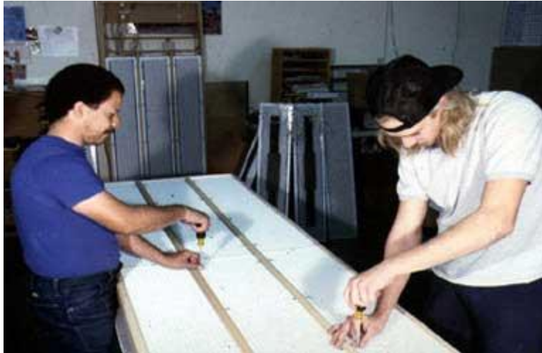
The panels are bolted into the wooden frame. A Spectra 6600 is shown.
