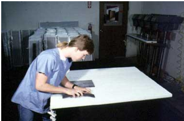
The felt dampening pads are glued to the rear of the completed panel, using the same contact adhesive.
