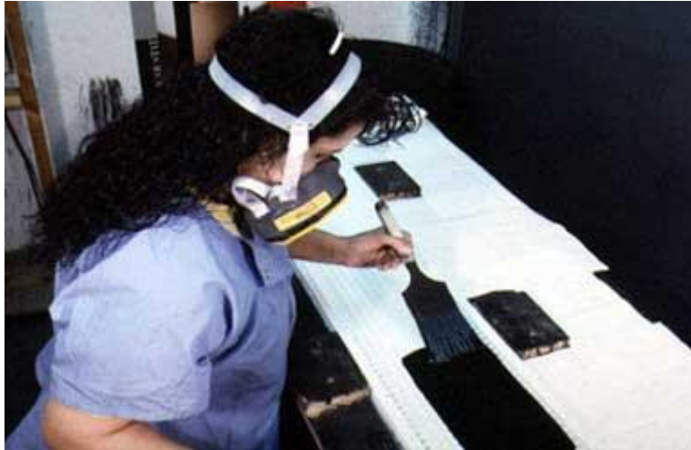
The conductive coating is hand-brushed onto the Mylar surface. The conductive coating is a proprietary mixture of several solvents, dissolved plastics, and carbon black.
