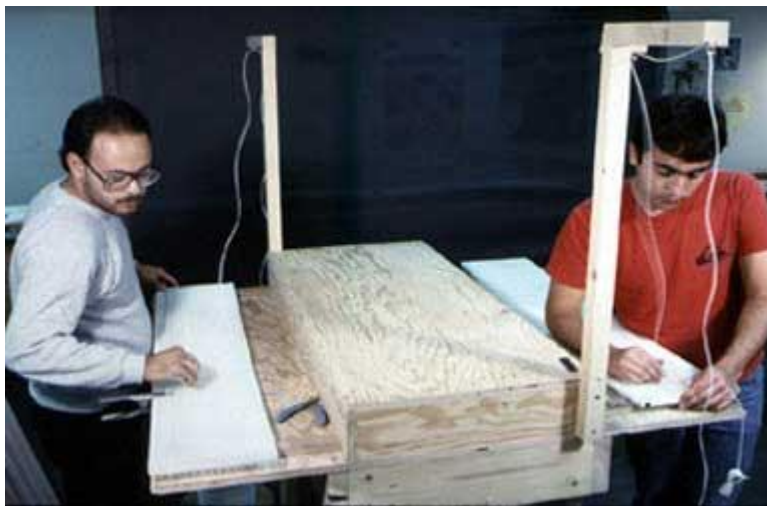
The louver is clamped in a slightly concave shape (curved toward the wire side) and strung with wires end-to-end over the entire surface.
