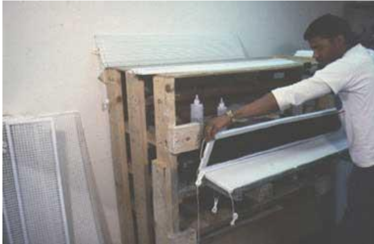
Special clamping fixtures are used to glue the two halves of the panel (one with Mylar, the other without) to form the finished panel. An industrial contact adhesive is used for this step.
