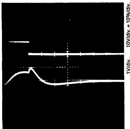
**PHOTO 1:**  $C_{test} = 10\mu F$ , 10V aluminum electrolytic;  $C_{ref} = 8\mu F$ , 200V polypropylene;  $R_L = 450\Omega$ ; residue  $\approx 12$  percent; 20msec pulse.
