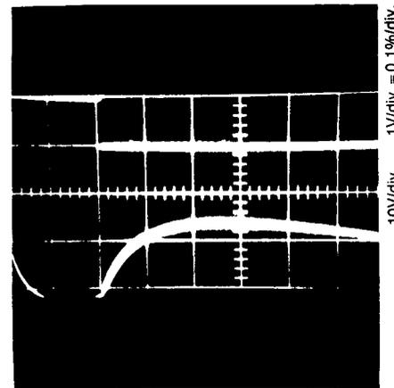
**PHOTO 6:**  $C_{test} = 10\mu F$ , 10V aluminum electrolytic;  $C_{ref} = 8\mu F$ , 200V polypropylene;  $R_L = 50k\Omega$ ; residue  $\approx 0.19$  percent; 20msec pulse.
