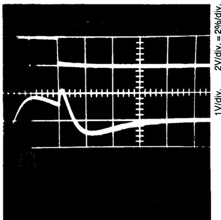
**PHOTO 2:**  $C_{test} = 10\mu F$ , 25V nonpolar aluminum electrolytic;  $C_{ref} = 8\mu F$ , 200V polypropylene;  $R_L = 500\Omega$ ; residue  $\approx 3$  percent; 20msec pulse.
