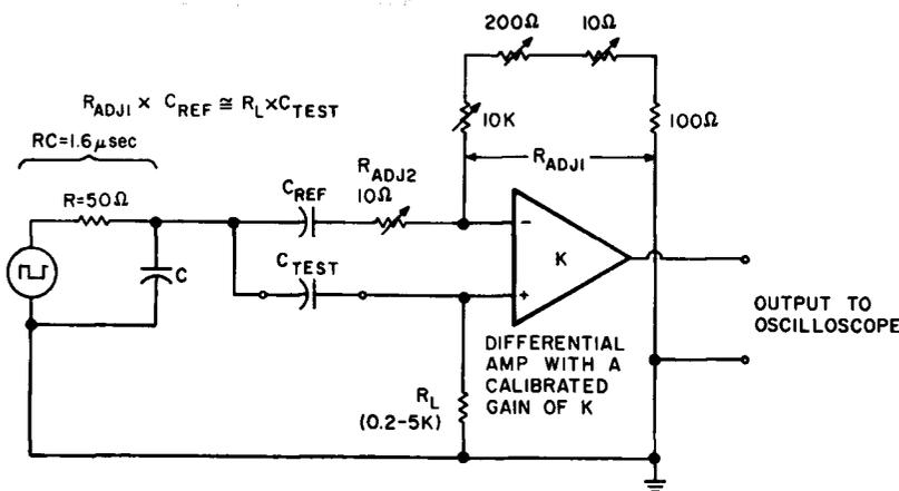
**FIGURE 1:** The basic test setup uses two RC networks and a calibrated differential amplifier. Trim  $R_{adj1}$  for coarse null. Trim  $R_{adj2}$  for fine null.  $C_{ref}$  should be reference-quality caps (Teflon are preferred, but polypropylene are adequate).
