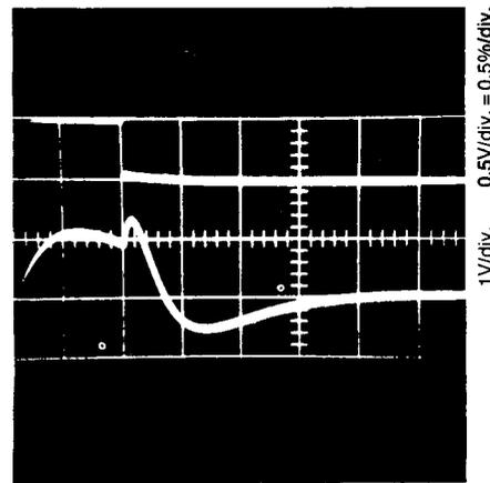
**PHOTO 3:**  $C_{test} = 10\mu F$ , 35V tantalum electrolytic;  $C_{ref} = 8\mu F$ , 200V polypropylene;  $R_L = 500\Omega$ ; residue  $\approx 0.9$  percent; 20msec pulse.
