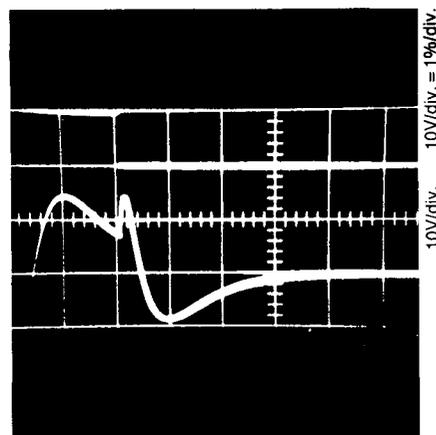
**PHOTO 4:**  $C_{test} = 0.1\mu F$ , 50V ceramic disk;  $C_{ref} = 0.1\mu F$ , 200V polypropylene;  $R_L = 50k\Omega$ ; residue  $\approx 2.4$  percent; 20msec pulse.
