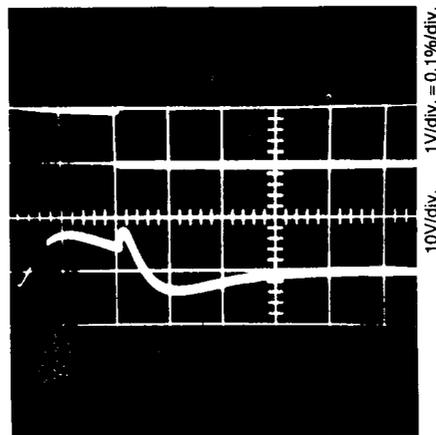
**PHOTO 5:**  $C_{test} = 0.1\mu F$ , 100V polyester (Mylar);  $C_{ref} = 0.1\mu F$ , 200V polypropylene;  $R_L = 50k\Omega$ ; residue  $\approx 0.11$  percent; 20msec pulse.
