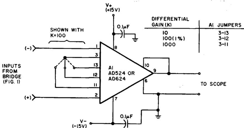
**FIGURE 2:** This selectable-gain differential preamp uses an IC instrumentation amp to realize the differential gain/level shift function.
