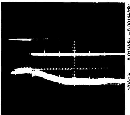
**PHOTO 7:**  $C_{test} = 1\mu F$ , 200V polystyrene;  $C_{ref} = 1\mu F$ , 50V Teflon;  $R_L = 10k\Omega$ ; residue  $\approx 0.001$  percent; 20msec pulse.
