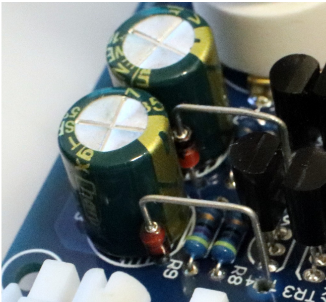
Zener diodes populated (used stashed 28V Zener diodes, 68k in parallel to get ~33k)
