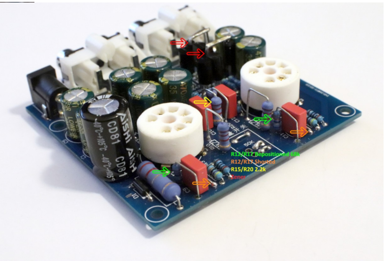
Zeners populated (used stashed 22V in series with 5.6V Zener diodes)
