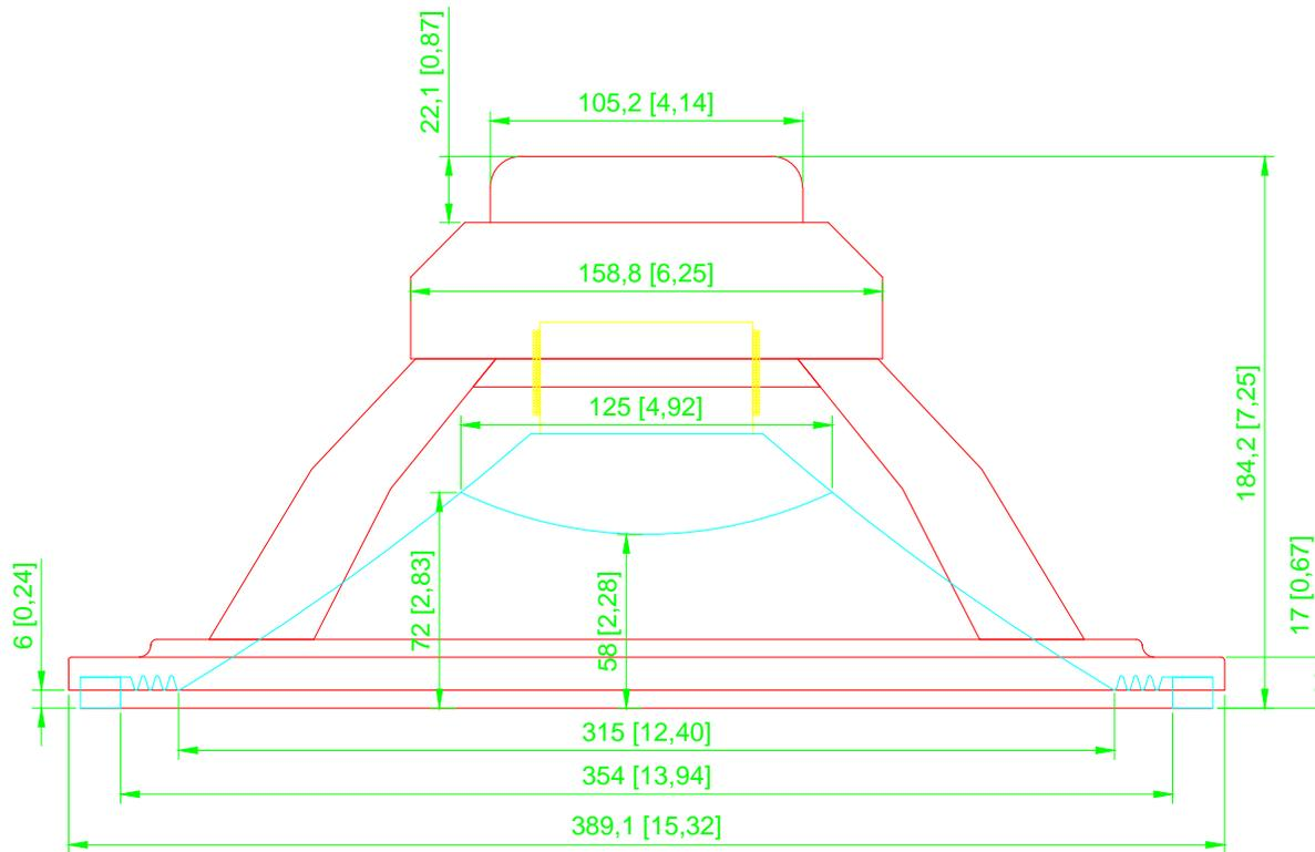
Eminence 3015LF, side view, scaled to data sheet overall diameter and depth.
