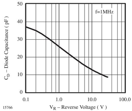
Figure 5. Typ. Diode Capacitance vs. Reverse Voltage
