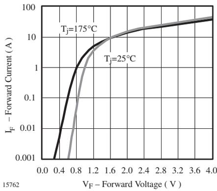
Figure 4. Max. Forward Current vs. Forward Voltage
