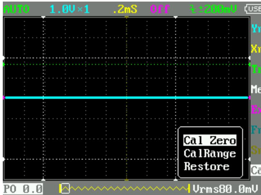
4. The calibration after the zero line, we need to save the Settings after calibration. By "+" or "-" button to move the cursor option "Yn" option, long press ">||" button, the pop-up "Save ParamTab?" window, press the ">||" button to save the calibration.
