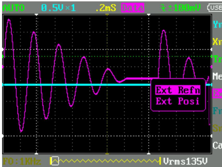
Set the cursor to the "EX" option, press the "M" pop-up window, select "Ext Refn" option, then Through "|<<" or ">>|" change cursor blink parameter values for the "Off", the two waveform operation line (purple line)Be hidden, as shown in the figure below.
