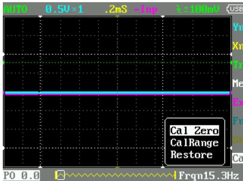
Oscilloscope Calibration: Press >||
