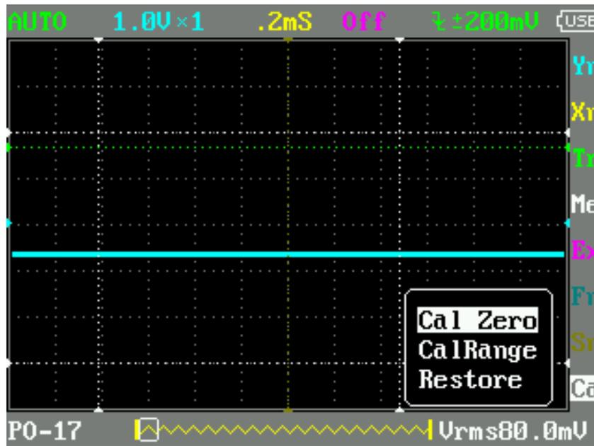
3. Select "Cal Zero" option, by "<<or">>" change the cursor blink in the parameter value is adjusted for "PO 0.0" Zero calibration line, line with the arrow to a level.
